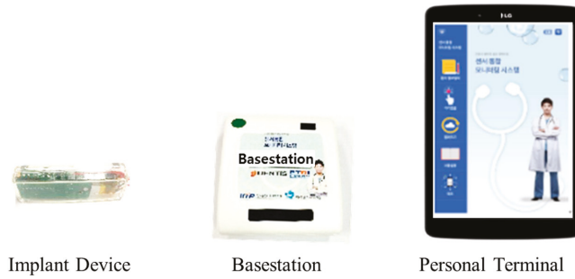
Figure 2. Developed prototype modules of the ECG monitoring system.
