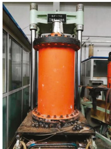
Figure 4. Large-scale triaxial shear test.
