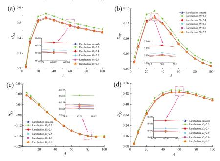
**Figure 17.** Effect of bearing number on dynamic damping coefficients with different fractal dimensions. (a)  $D_{xx}$  vs.  $\Lambda$ ; (b)  $D_{xy}$  vs.  $\Lambda$ ; (c)  $D_{yx}$  vs.  $\Lambda$ ; (d)  $D_{yy}$  vs.  $\Lambda$ .
