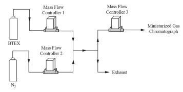
Figure 3. Experimental setup for BTEX generation.
