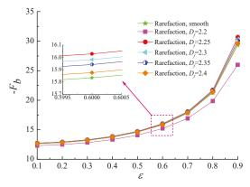
**Figure 8.** Static friction coefficient versus eccentricity ratio for different fractal dimensions at  $\Lambda$  = 20, G = 1  $\times$  10<sup>-11</sup>.
