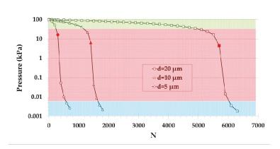
**Figure 8.** Inlet pressure evolution of a system connected to pump B as a function of its number of stages, considering narrow diameter channels  $d=5,10,20~\mu m$  and a constant outlet pressure  $P_{out}=100~k Pa$  (red solid symbols represent the pressure and stage number, where the maximum slope, corresponding to the peak values of Figure 5a, is observed).
