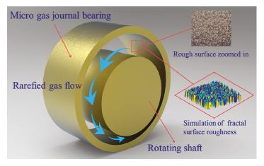
Figure 2. Schematic of a rough-surface gas-lubricated journal microbearings.
