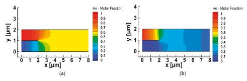
**Figure 6.** Molar fraction of He in the micro-mixer imposing: (a) equal inlet pressures of He and Xe, and (b) equal inlet fluxes of He and Xe.
