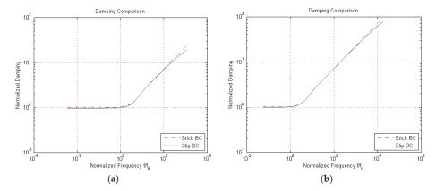
**Figure 7.** Engaged solution, (a)  $H = 3 \,\mu\text{m}$  and (b)  $H = 12 \,\mu\text{m}$ : normalized damping at varying frequency f, for both stick and slip BCs.
