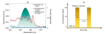
**Figure 2.** (a) Absorption spectra of toluene (100 ppm), background gas, i.e., nitrogen, and emission spectrum of deep UV-LED. (b) Schematics of flushing routine of nitrogen and toluene for measuring reference and measured intensity respectively.
