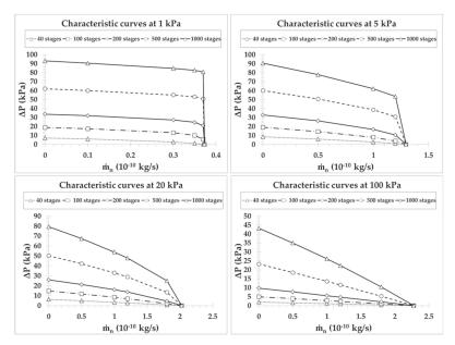
**Figure 10.** Performance characteristic curves of a Knudsen pump, based on pump C, for a number of stages N=40,100,200,500,1000 with inlet pressures  $P_{in}=1,5,20,100$  kPa when narrow microchannels diameter d=10 μm and wide channel diameter D=100 μm.
