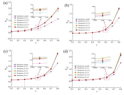
**Figure 14.** Effect of eccentricity ratio on dynamic stiffness coefficients with different fractal dimensions. (a)  $K_{xx}$  vs.  $\varepsilon$ ; (b)  $K_{xy}$  vs.  $\varepsilon$ ; (c)  $K_{yx}$  vs.  $\varepsilon$ ; (d)  $K_{yy}$  vs.  $\varepsilon$ .
