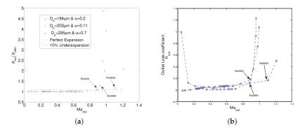
**Figure 9.** flow choking and underexpansion for simulated MCs: back pressure (a), and  $K_{out}$  (b).
