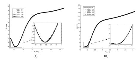
**Figure 3.** Grid independence study by analysing the slip velocity distribution on the bottom wall. Legends show the number of cells in x direction (along the length of channel)  $\times y$  direction (along the height of channel). (a) Kn = 0.01; (b) Kn = 0.05.
