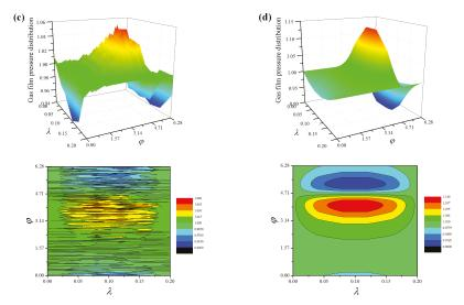
**Figure 5.** Pressure distributions and contour plots of the gas-lubricated microbearing for different bearing numbers and eccentricity ratios: (a)  $\varepsilon = 0.6$ ,  $\Lambda = 20$ ,  $D_f = 2.3$ , and  $G = 1 \times 10^{-10}$  m, (b)  $\varepsilon = 0.6$ ,  $\Lambda = 60$ ,  $D_f = 2.3$ , and  $G = 1 \times 10^{-10}$  m, (c)  $\varepsilon = 0.3$ ,  $\Lambda = 20$ ,  $D_f = 2.3$ , and  $G = 1 \times 10^{-10}$  m, and (d)  $\varepsilon = 0.6$ ,  $\Lambda = 20$ , smooth.
