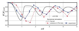
**Figure 4.** Comparison of the experimental and predicted data for a real microjet escaping from the nozzle  $16.1 \mu m$  in diameter at n = 2.04.
