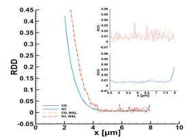
Figure A1. Distribution of relative density difference of CO and  $N_2$  calculated with the present definition and Wang and Li's definition in [15]; the results are zoomed for a specific channel length at the upper right.
