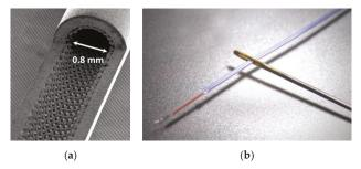
**Figure 1.** Microstructure fluidic device. (a) Micro heat pipe, opened to see the inside structure. Inner diameter is 0.8 mm. From: KIT-IMVT; (b) Miniaturized Type K thermocouple. Although this sensor has an outer diameter of 0.4 mm only, a major part of the structure in (a) would have been blocked. Picture from: www.ninomiya-ew.co.jp.
