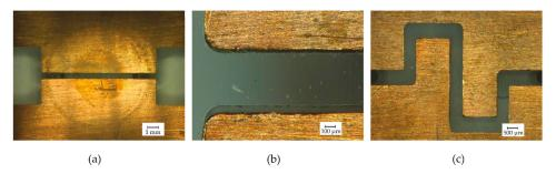
**Figure 7.** Digital optical microscope images of copper electrodes assembled on bottom polymethyl methacrylate (PMMA). (a) Channel 1; (b) Zoom at bottom PMMA and copper electrodes assembly; (c) Channel 2.
