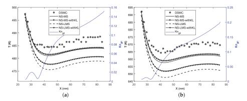
**Figure 10.** Temperature distribution of the fluid on the bottom wall at Kn = 0.01. (a)  $T_w = 500 \text{ K}$ ; (b)  $T_w = 700 \text{ K}$ .
