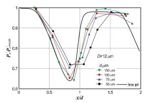
Figure 5. Calculated impingement of jets escaping from nozzles of different diameters onto the Pitot tube  $12 \mu m$  in diameter.
