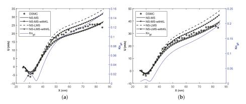
Figure 11. Velocity slip distribution on the bottom wall at Kn = 0.01. (a)  $T_w = 500 \text{ K}$ ; (b)  $T_w = 700 \text{ K}$ .
