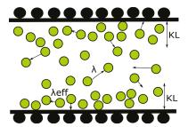
**Figure 1.** Schematic of inter-molecular and molecule-surface collisions leading to the formation of Knudsen layer (KL).
