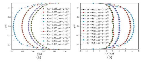
**Figure 4.** Calculation results of different time steps. (a) Velocity distributions on the outlet of the narrow channel; (b) temperature distributions on the outlet of the narrow channel.
