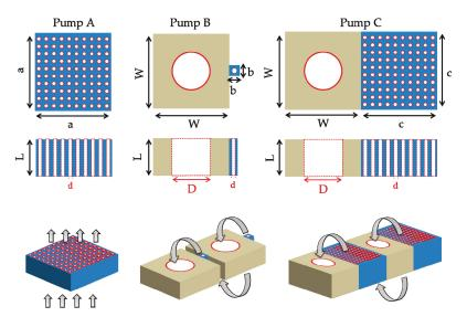
**Figure 1.** Representative view of single-stage pump A, and of two consecutives stages of multistage pumps B and C. Gray arrows denote the pumping flow direction, the hot and cold regions being at the top and the bottom of each stage, respectively.
