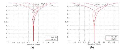
**Figure 6.** Engaged solution, (a)  $H = 3 \mu m$  and (b)  $H = 12 \mu m$ : snapshots of the velocity profile during a single cycle of oscillation of the plate at y = H, for  $f = 100 f_d$  and both stick and slip BCs.
