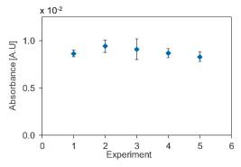
**Figure 6.** Absorbance for different experimental conditions for repeatability and reproducibility. (1) flowrate, 40 mL/min; (2) flowrate, 20 mL/min; (3) flowrate, 10 mL/min; (4) Detector integration time, 50 ms; and (5) LED current input, 15 mA.
