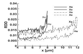
Figure 4. Detailed view of the evolution of the relative density difference of He and Xe in the downstream part of the mixing zone of micro-mixers with a total length of 8  $\mu$ m (solid grey) and 12  $\mu$ m (dash-dot black).
