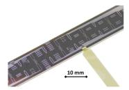
**Figure 2.** Silicon microstructure chip for temperature measurement in a gas flow. The chip is inserted into a sealed housing and forms the fourth side of a rectangular microchannel. Numerous thermopiles have been implemented into the chip, to measure the temperature of a gas flow in combination with precision resistors [78]. www.gasmems.eu.
