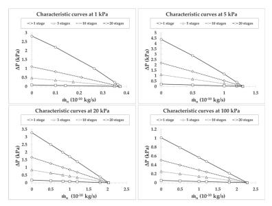
**Figure 9.** Performance characteristic curves of a Knudsen pump, based on pump C, for a number of stages N=1,5,10,20 with inlet pressures  $P_{in}=1,5,20,100$  kPa when narrow microchannels diameter d=10 μm and wide channel diameter D=100 μm.
