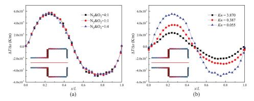
Figure 6. Temperature gradient on the central axis of the channel. (a) Kn = 0.055; (b)  $N_2$  and  $O_2 = 4:1$ .
