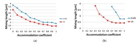
**Figure 5.** Mixing length variation over different accommodation coefficients  $\alpha$  at walls: (a) all walls have the same  $\alpha \in [0,1]$  and (b) the upper wall has  $\alpha \in [0,1]$ , while all other walls have  $\alpha = 1$ .
