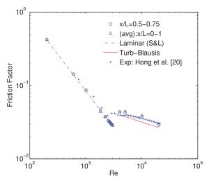
Figure 5. Numerical validation of friction factor calculation.
