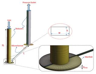
Figure 4. Details of numerical model and meshing.
