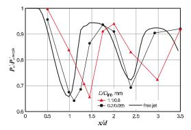
Figure 6. Calculation of the model microjet escaping from the nozzle 1.06 mm in diameter (modeling exhaustion from the nozzle 16.1  $\mu$ m in diameter) and impinging onto the Pitot tubes of different diameters.
