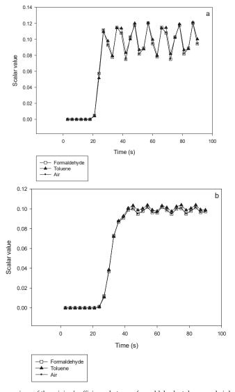
**Figure 8.** Comparison of the mixing's efficiency between formaldehyde, toluene and air being mixed with pure air at  $25 \text{ NmL} \cdot \text{min}^{-1}$ . Variations of the scalar value with time at the exit of a 2-stages (a) or 4-stages (b) device, illustrating that there is almost no time response difference between formaldehyde, toluene and air.
