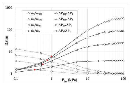
**Figure 4.** Ratios of total maximum mass flow rates  $\dot{m}_1/\dot{m}_n$  and associated maximum pressure differences  $\Delta P_n/\Delta P_1$  for various one-stage layouts (numbers of microchannels n=4,25,100,400 and corresponding diameters d=50,20,10,5 µm) compared to the reference layout (n=1,d=100 µm).
