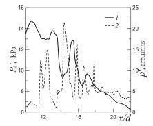
**Figure 13.** Pitot pressure  $P_0$ ′ (solid curve 1) and amplitude of acoustic oscillations p′ of mode B (dotted curve 2) versus the normalized distance from the nozzle; d = 0.72 mm, D = 0.4 mm, and n = 3.
