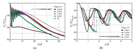
Figure 7. Pressure distribution in the jet escaping from the nozzle 1.06 mm in diameter (modeling exhaustion from the nozzle 16.1  $\mu$ m in diameter). The plots in (b) are fragments from (a).
