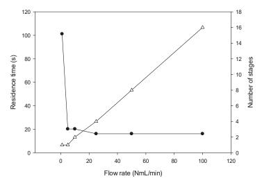
Figure 7. Number of stages ( $\Delta$ ) required for the oscillations of the scalar value at the micromixer's exit to be lower than 5% of the targeted value 0.1 at flow rates ranging from 1 to 100 NmL·min<sup>-1</sup>. Variations of the residence time ( $\bullet$ ) with the flow rate for the corresponding number of stages required. At 100 NmL·min<sup>-1</sup>, the 5% threshold is not reached: the percentage of oscillations is 6.1% after the 16th stage of mixing.
