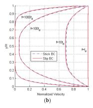
**Figure 3.** Disengaged solution, (a)  $H = 3 \, \mu m$  and (b)  $H = 12 \, \mu m$ : maximum amplitude of the velocity profile at varying frequency f of oscillation of the two plates, for both stick and slip boundary conditions (BCs).
