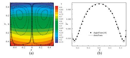
**Figure 3.** The simulation results of square cavity with dsmcFoam. (a) Temperature contours and velocity streamlines at Kn = 0.1 by dsmcFoam. (b) Profile of the V component of the velocity on horizontal line, passing through the center of the left primary vortex at Kn = 0.1. In (b), black points show the results extracted from [43], and the curve shows the results of dsmcFoam.
