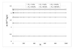
**Figure 7.** Maximum mass flow rate (corresponding to zero pressure difference) of pump B with single narrow and wide microchannels of diameters  $d=10~\mu m$  and  $D=100~\mu m$ , respectively, in each stage, at various inlet pressures, versus the number of stages.
