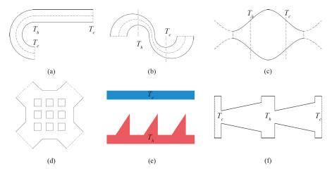
**Figure 1.** Common Knudsen pump channel structures: (a) Curve-straight channel, (b) double-curves channel, (c) sinusoidal channel, (d) matrix channel, (e) ratchet channel, (f) taper channel.
