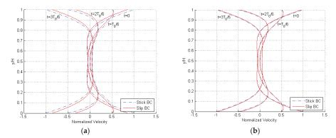
Figure 4. Disengaged solution, (a)  $H = 3 \mu m$  and (b)  $H = 12 \mu m$ : snapshots of the velocity profile during a single cycle of oscillation of the two plates, for  $f = 100 f_d$  and both stick and slip BCs.
