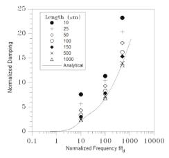
Figure 9.  $H=3~\mu m$ , disengaged solution, stick BCs: effect of surface length on the normalized damping value.
