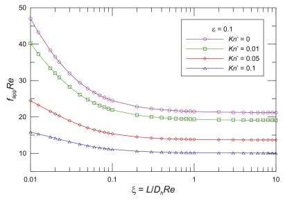
**Figure 2.** Effect of  $Kn^*$  on  $f_{app}Re$  for rectangular ducts ( $\varepsilon = 0.1$ ).
