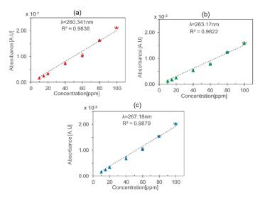
Figure 4. Absorbance vs. toluene concentration using the glass HCW at different wavelengths: (a)  $\lambda_1 = 260.34$  nm, (b)  $\lambda_2 = 263.17$  nm, (c)  $\lambda_3 = 267.18$  nm. The vertical and the horizontal error bars represent standard deviations in absorbance values and combined uncertainties in the generated concentrations defined by the uncertainties of mass flow controllers (MFCs) and gas cylinder concentrations, respectively.
