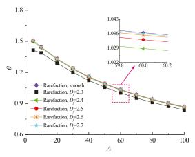
**Figure 10.** Attitude angles versus bearing number for different fractal dimensions at ε = 0.6,  $G = 1 \times 10^{-10}$ .
