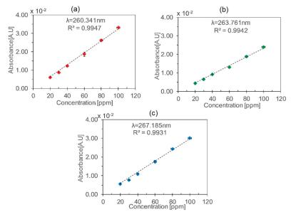
Figure 5. Absorbance vs. toluene concentration using the aluminium HCW at different wavelengths: (a)  $\lambda_1 = 260.34$  nm, (b)  $\lambda_2 = 263.17$  nm, and (c)  $\lambda_3 = 267.18$  nm. The vertical and the horizontal error bars represent standard deviations in absorbance values and combined uncertainties in the generated concentrations defined by the uncertainties of MFCs and gas cylinders, respectively.
