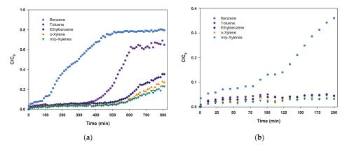
**Figure 5.** (a)  $C/C_0$  vs. time during a breakthrough experiment performed with an equimolar 1 ppm mixture of BTEX over Basolite-filled preconcentrator and (b) enlarged view of the first 200 min of the experiment.
