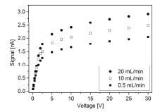
**Figure 8.** Channel 3 signal with variation of voltage on copper electrodes for various gas sample flow-rates. Uncertainty bars are not displayed in the graphic since their size is small compared to the symbols representing the points.
