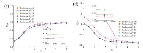
Figure 13. Effect of perturbation frequency on dynamic damping coefficients with different fractal dimensions. (a)  $D_{xx}$  vs.  $\Omega$ ; (b)  $D_{xy}$  vs.  $\Omega$ ; (c)  $D_{yx}$  vs.  $\Omega$ ; (d)  $D_{yy}$  vs.  $\Omega$ .
