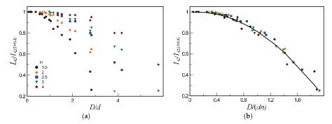
**Figure 8.** Normalized length of the supersonic core of the jet versus the ratio of the Pitot tube and nozzle diameters (**a**) and versus the ratio of the Pitot tube diameter D and nozzle diameter d multiplied by n (**b**).
