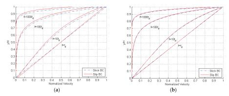
**Figure 5.** Engaged solution, (a)  $H = 3 \mu m$  and (b)  $H = 12 \mu m$ : maximum amplitude of the velocity profile at varying frequency f of oscillation of the moving plate at y = H, for both stick and slip BCs.
