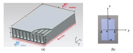
**Figure 1.** Schematics of the microchannel plate fin heat sink. (a) Microchannel plate fin heat sink; (b) Computational unit.
