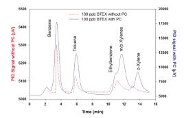
Figure 8. Red dashed line: Chromatogram of 100 ppb BTEX without preconcentration step (sample volume of 200  $\mu$ L). Blue solid line: Chromatogram of 100 ppb BTEX with preconcentration step (sample volume of 20 mL).
