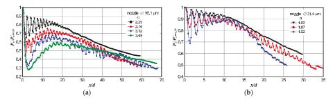
Figure 9. Pressure distributions in real microjets escaping from nozzles 21.4 (a) and 16.1  $\mu$ m in diameter (b).
