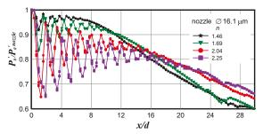
**Figure 2.** Axial pressure distribution measured by the Pitot tube in the jet escaping from the nozzle 16.1 µm in diameter.
