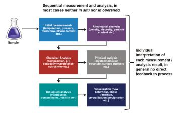
**Figure 6.** Current state-of-the-art sequential measurement and analysis method. The timely and locally separated measurement makes it difficult or even impossible to correlate measurement results to each other and retrieve by this deeper insight into the underlying mechanisms.
