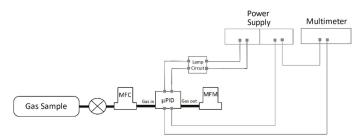
Figure 6. Experimental setup used for signal measurements from  $\mu$ PID prototype.
