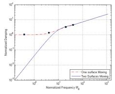
Figure 8.  ${\it H}=3~\mu m$ , stick BCs: comparison between the values of normalized damping for engaged and disengaged solutions.
