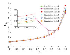
Figure 6. Non-dimensional load capacity versus eccentricity ratio for different fractal dimensions at  $\Lambda = 20$ ,  $G = 1 \times 10^{-11}$ .
