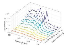
**Figure 3.** Absorbance of toluene at different wavelengths for different concentrations of toluene using the glass hollow core waveguide (HCW).
