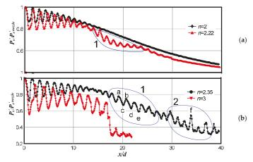
**Figure 10.** Pressure distribution in the model microjet escaping from the nozzle 1.06 mm in diameter (modeling exhaustion from the nozzle 16.1  $\mu$ m in diameter). (a) n = 2 and 2.22, (b) n = 2.35 and 3.
