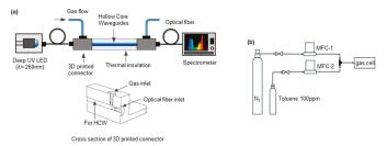
Figure 1. (a) Experimental setup for toluene detection. (b) Toluene concentration generation setup.
