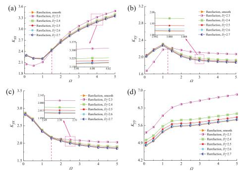
**Figure 12.** Effect of perturbation frequency on dynamic stiffness coefficients with different fractal dimensions. (a)  $K_{xx}$  vs.  $\Omega$ ; (b)  $K_{xy}$  vs.  $\Omega$ ; (c)  $K_{yx}$  vs.  $\Omega$ ; (d)  $K_{yy}$  vs.  $\Omega$ .
