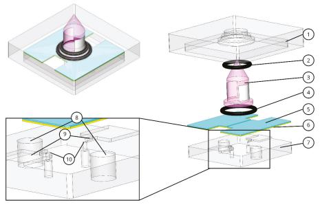
**Figure 1.** Assembled and exploded view of the detector core. (1) Top poly(methyl methacrylate) (PMMA), (2) O-ring 1, (3) UV lamp, (4) O-ring 2, (5) shield, (6) copper electrodes, (7) bottom PMMA, (8) electrode connection holes, (9) elevation structure, (10) micro-pores.
