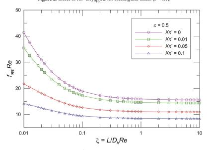
**Figure 3.** Effect of  $Kn^*$  on  $f_{app}Re$  for rectangular ducts ( $\varepsilon = 0.5$ ).
