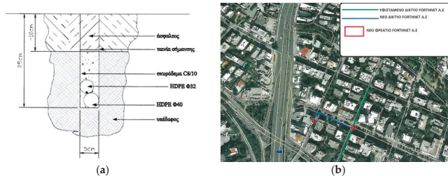
Figure 1. Documentation submitted for granting rights of way for public utilities. (a) Typical cross section; (b) location of network lines on drawing [23].
