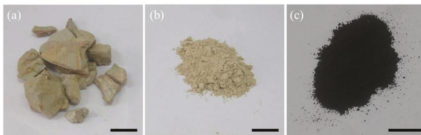
**Figure 1.** Digital camera images of (a) the crude mineral ore of attapulgite (ATP), (b) purified ATP and (c) the ATP/polypyrrole (PPy) nanocomposite. Scale bar: 1 cm.
