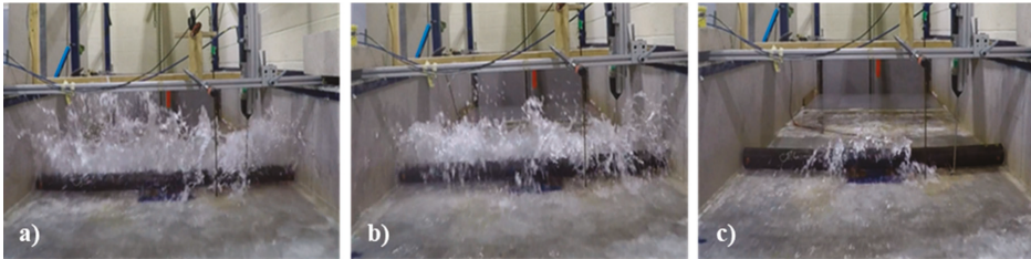
Figure 7. Bore impact on the pipe for three impoundment depths: (a) h = 50 cm, (b) h = 40 cm, and (c) h = 30 cm.
