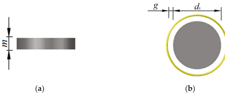
Figure 6. Parameters of the silicon rod (a) Front view; (b) Top view.
