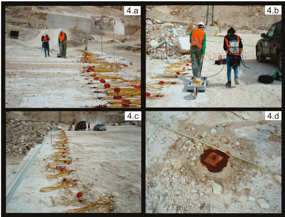
Figure 4. (a) GPR profile performed on the marble bench; (b) Detail from the 250 MHz antenna on the bank; (c) Position of the ERI profile on the primary bank; (d) Detail of a copper electrode and clay.
