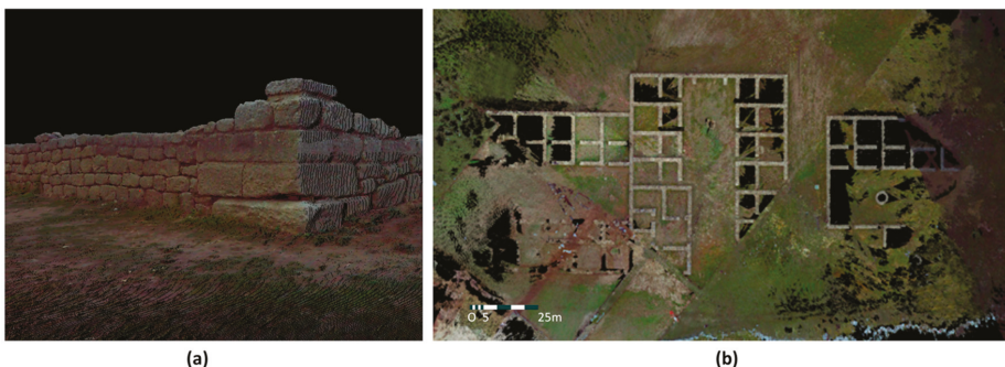
Figure 6. Results of the T-LiDAR survey: (a) Detailed view of a colored 3D point cloud of a stone wall and (b) orthoimage of the barrack in the Southern area of the Roman site.
