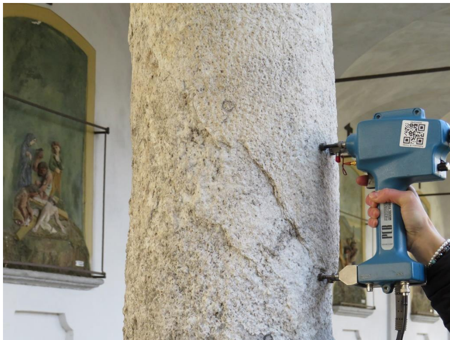
Figure 8. Impact test carried out on a column of Via Crucis portico.
