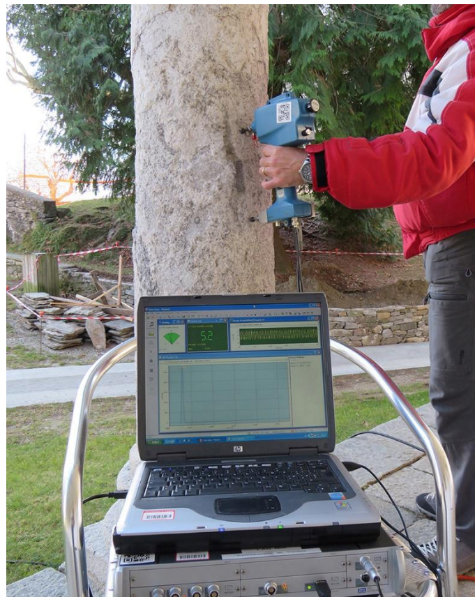
Figure 5. Setup of the impact test.
