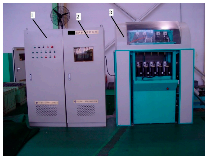
Figure 5. Appearance of testing equipment (1. PLC control unit; 2. PC control unit; 3. mechanical device).
