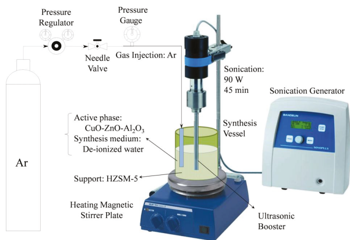
Figure 13. Experimental setup for dispersion of CZA over HZSM-5 using US energy. Reprinted from Ref. [90]. Copyright 2014 with permission of The Royal Society of Chemistry.
