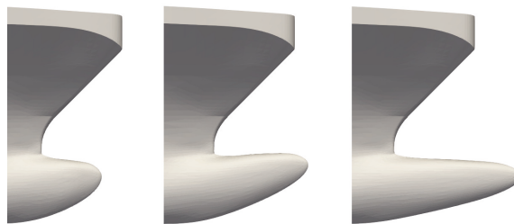
Figure 15. Bulbous bow shapes. Left: original shape. Middle: shape obtained at global minimum. Right: shape obtained at local minimum.
