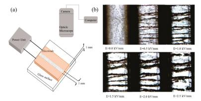
**Figure 10.** (a) Schematic illustration of polarizability measuring device; (b) optical microscope (OM) images showing the polarization of nanocube-TiO<sub>2</sub>/poly(3-octhlthiophene)-based ER fluid, reprinted with permission from [104]. Copyright John Wiley and Sons, 2016.
