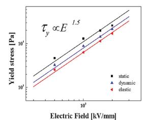
Figure 12. Static, dynamic, and elastic yield stresses as a function of electrical field strength for PANI-nanotube-based ER suspension, reprinted with permission from [119]. Copyright Elsevier, 2017.
