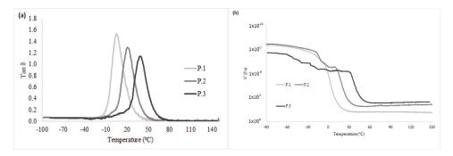
Figure 7. DMTA thermograms of the synthesized PUs. (a) Loss factor; (b) Storage modulus.
