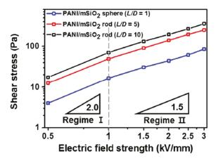
**Figure 14.** Yield stress of PANI/mSiO<sub>2</sub>-based ER suspension as a function of electrical field strength, reprinted with permission from [127]. Copyright Elsevier, 2016.
