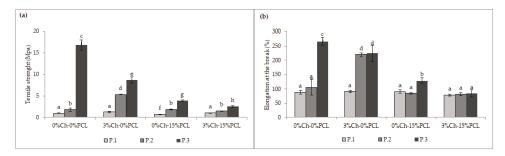
**Figure 1.** Mechanical properties of the synthesized PUs. (a) Maximum stress of PUs; (b) Percent elongation of PUs. The data are expressed as the mean  $\pm$  SD (n = 3). Bars with different letters (a–h) indicate significant differences (p < 0.05) between the polyols.
