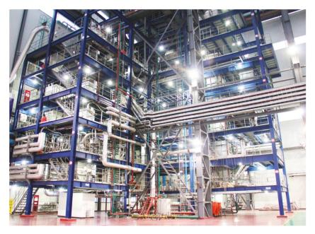
Figure 3. Dongfang boiler 3-MW circulating fluidized bed combustion test bench.
