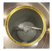
Figure 5. The cup ignition test with two thermocouples.
