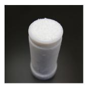
Figure 1. A typical sample of methane hydrate while in the Teflon cylindrical mold.
