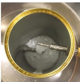
**Figure 5.** The cup ignition test with two thermocouples.
