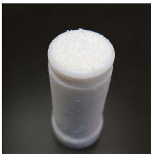
**Figure 1.** A typical sample of methane hydrate while in the Teflon cylindrical mold.
