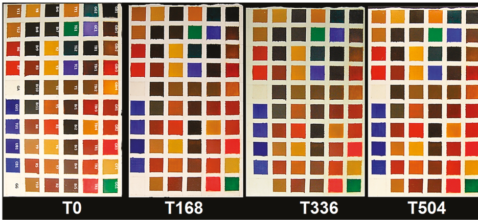
Figure 6. Full colour RGB (red, green and blue) images of the sample set at the different ageing times.
