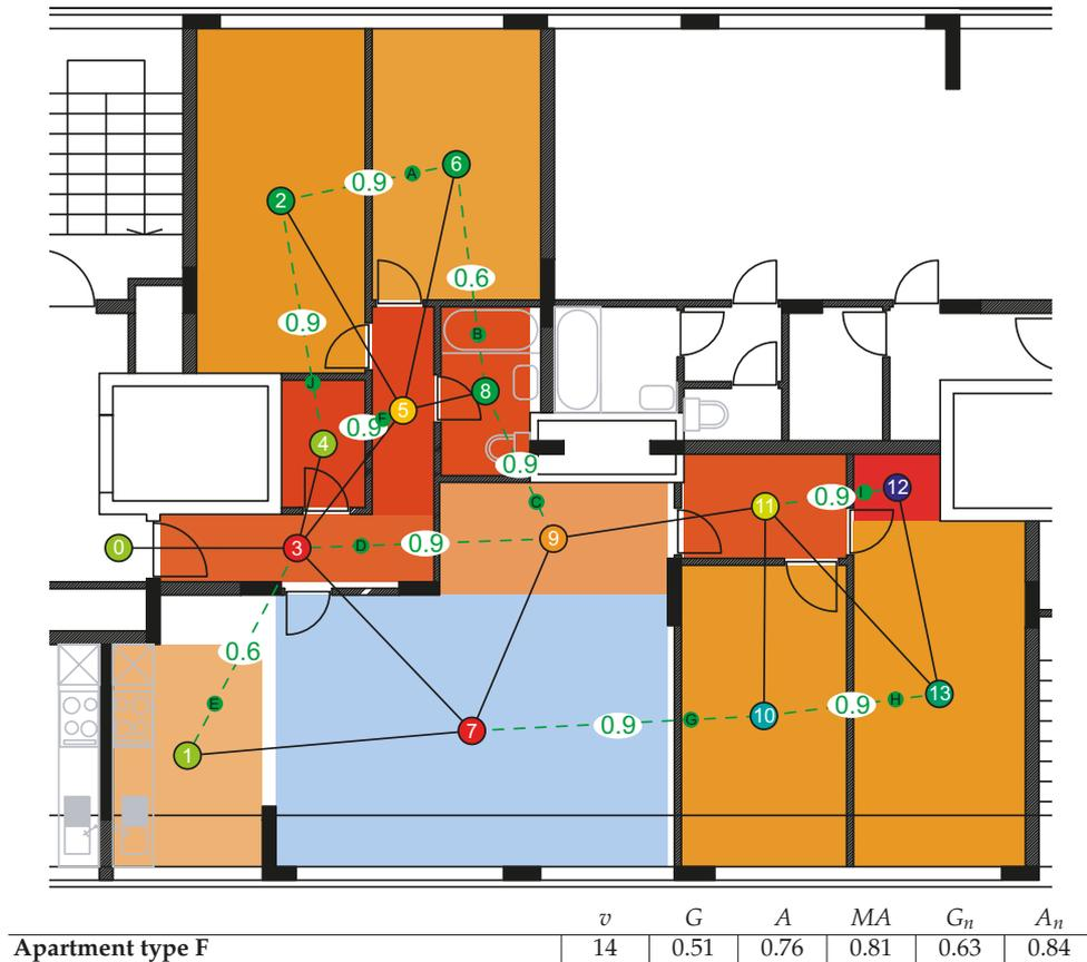
Figure 6. SAGA analysis of apartment type F.
