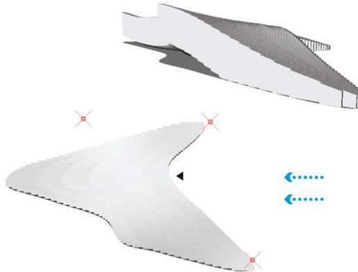
**Figure 10.** The third set of variable parameters. The floor plan depicting shape-influencing points (red) and wind direction (blue arrows).
