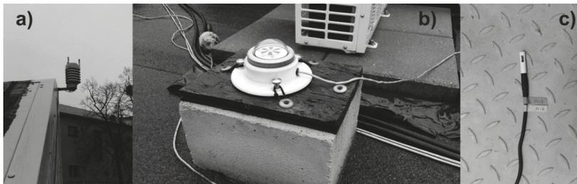
**Figure 1.** Measuring equipment, instruments for measuring environmental values: (a) weather station; (b) pyranometer; and (c) temperature sensor and relative humidity of the air [28,29].
