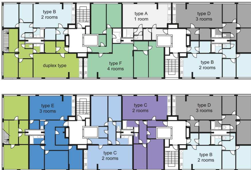
**Figure 4.** Overview of the seven unit types in Paduart’s refurbishment proposal. Image by Paduart [36], used with permission.
