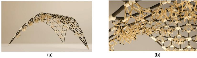
**Figure 1.** Carrier component structure: (a) detailed design of a discrete carrier surface as a support structure; and (b) aggregation of a single adaptive component over the surface.
