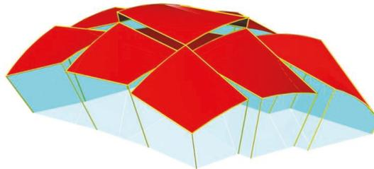
**Figure 19.** Visualization of another modified free form structure roofed with a multi-segment shell structure and folded elevation.
