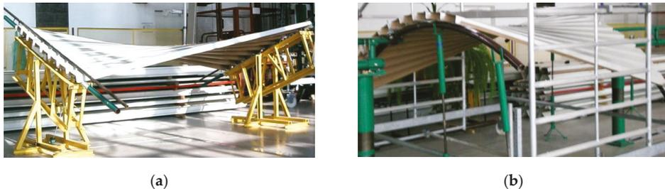
**Figure 3.** Experimental transformed corrugated shells supported by: (a) straight directrices, (b) curved directrices.
