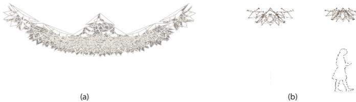
**Figure 2.** (a) Design rendition of responsive envelope on carrier surface; and (b) adaptive component triggering closed and open states through motion.
