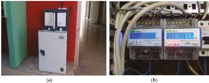
Figure 2. Experimental equipment for measurements of (a) IEQ and (b) electrical consumption within the building of B FEPA.
