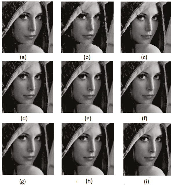
Figure 5. Results of different filters in restoring 40% corrupted Lena image: (a) adaptive switching median filter (ASWM); (b) tri-state median filter (TSM); (c) progressive switching median filter (PSM); (d) luo-iterative median filter (Luo); (e) directional weighted median filter (DWM); (f) Adaptive Switching Median Filter (ASWM); (g) Switching Bilateral Filter (SBF); (h) Robust Outlyingness Ratio Non-Local Mean (ROR-NLM); (i) proposed method.
