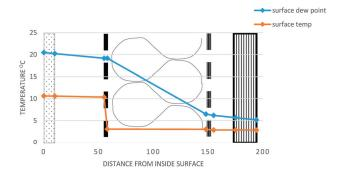
Figure 3. Interstitial condensation calculations in the test house.
