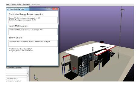
Figure 11. Energy analysis functionality in smart built environment.
