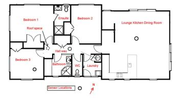
Figure 7. House plan with sensor locations.
