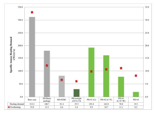
**Figure 5.** Comparison of specific annual heating demands (kWh/(m<sup>2</sup>a)) and overheating time (%) of the base case and different retrofitting packages.
