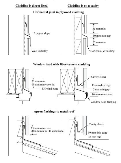
Figure 3. A selection of flashings used in NZ buildings and taken from E2/AS1.
