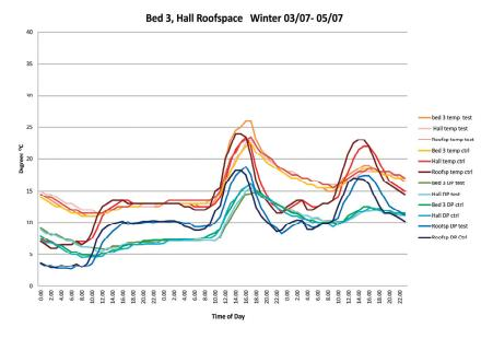
**Figure 13.** Dry bulb temperatures and dew point comparisons for the bedroom 3 hall and roofspace with external winter conditions.
