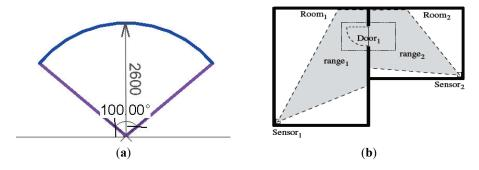
**Figure 3.** (a) Example of the range space of a sensor with range radius of 2.6 m and a range angle of 100°; (b) the door's operational space should be within the range space of the two monitoring sensors.
