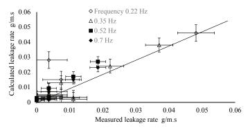
**Figure 8.** A comparison of measured and calculated leakage rates with fluctuating air pressures and showing experimental uncertainties.
