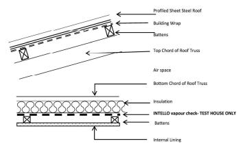
Figure 6. Construction detail—roof.
