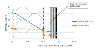
Figure 2. Interstitial condensation calculations in the control house.
