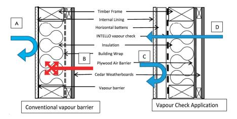
Figure 1. Moisture flows through the structure.
