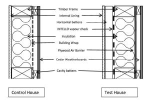
Figure 5. Construction detail—external walls.
