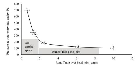
**Figure 11.** Pressure difference at the onset of leakage through a window head joint as a function of runoff rate over the joint.
