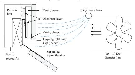
Figure 15. Experimental apron flashing joint between roof.
