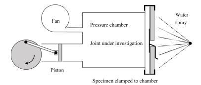
Figure 2. Equipment for measuring the weathertightness characteristics of joints.
