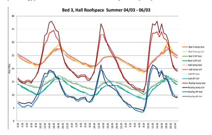
**Figure 12.** Dry bulb temperatures and dew point comparisons for the bedroom 3 hall and roofspace with external summer conditions.
