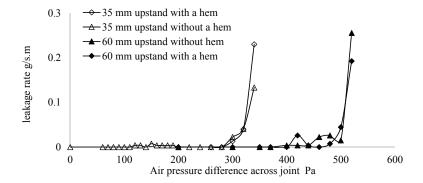
**Figure 6.** Steady pressure leakage characteristics of flashings with 35 and 60 mm upstands with and without hems.
