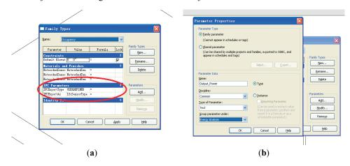
**Figure 2.** (a) Extending BIM design using the "IFC shared parameter"; (b) Adding new parameter properties in Revit.
