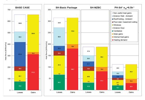
**Figure 7.** Heat flows (losses and gains) of the Base Case (axis maximum value: 700 kWh/(m<sup>2</sup>a)) and comparison of heat flows (losses and gains) of SH-BP, SH-NZBC and PH-S4\* (axis maximum value: 350 kWh/(m<sup>2</sup>a)) calculated with PHPP.
