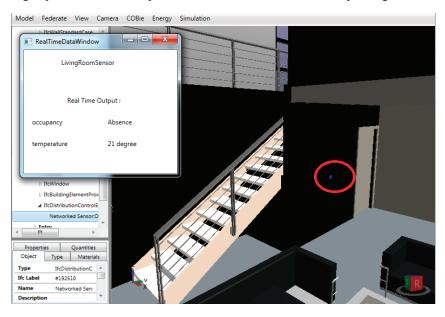
Figure 10. Real-time monitoring data display to the user.
