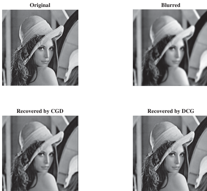
Figure 6. The original image (top left), the blurred image (top right), the restored image by CGD (bottom left) with SNR = 22.93, SSIM = 0.87 and by DCG (bottom right) with SNR = 24.36, SSIM = 0.90.
