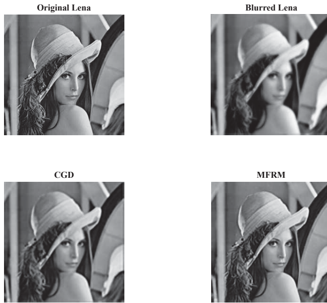
Figure 10. The original image (top left), the blurred image (top right), the restored image by CGD (bottom left) with time = 5.38, SNR = 25.97 and SSIM = 0.88, and by MFRM (bottom right) with time = 38.77, SNR = 26.26 and SSIM = 0.90.
