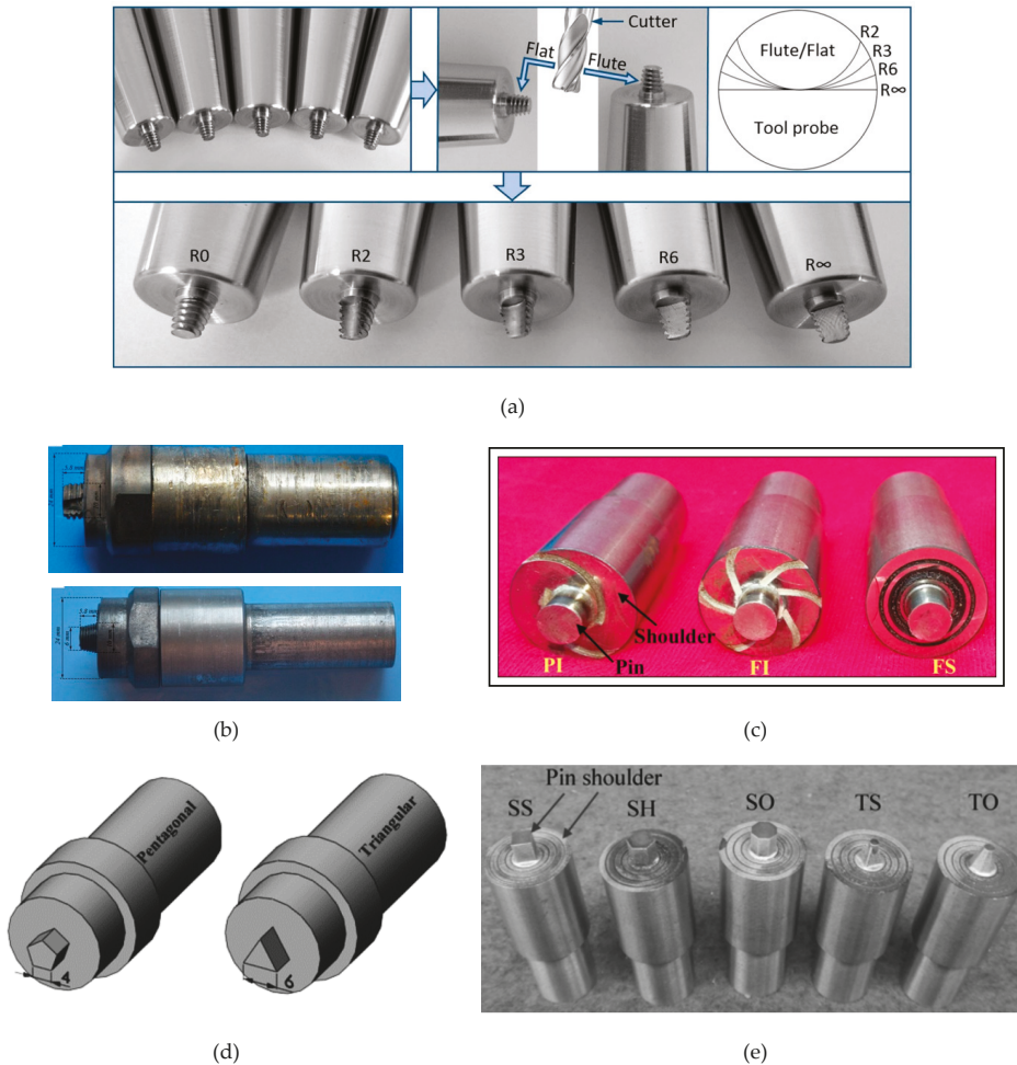
Figure 8. Tools of different geometries used in different Al alloy combinations. (a) AA2024-AA7075, reproduced from [14], with permission from Springer, 2018; (b) AA5083-AA7075, reproduced from [16], with permission from Springer, 2018; (c) AA5083-AA6351, reproduced from [18], with permission from SAGE, 2018; (d) AA5083-AA6082 [34], with permission from the authors; (e) AA5083-AA6351 [57], with permission from Springer, 2013.
