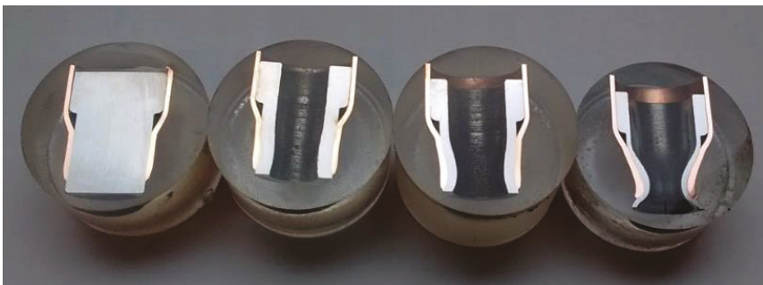
Figure 11. Metallographic specimens of typical welds: (left to right) Tube-to-rod, tube-to-tube with a target tube with a wall thickness of 3, 2 and 1 mm.
