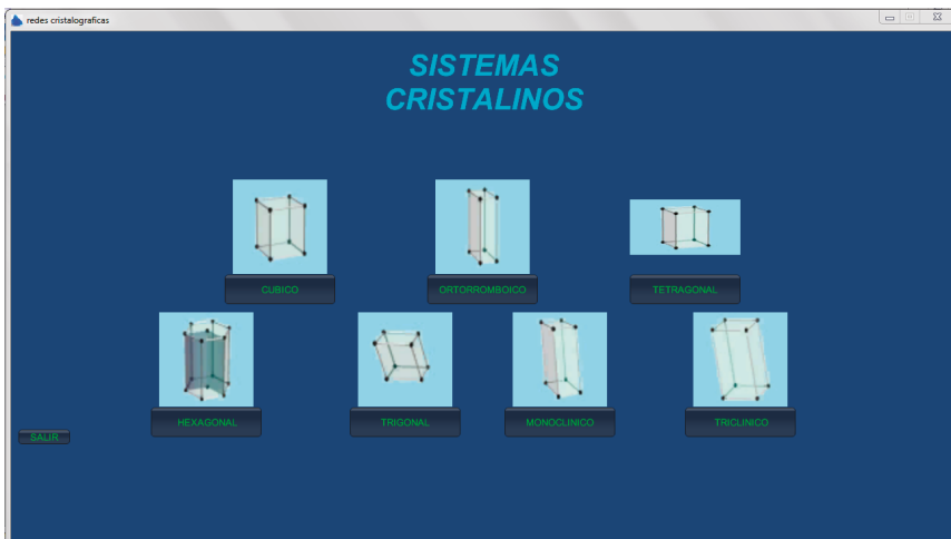
Figure 2. Main screen of the Didactic Virtual Tool showing the seven crystal systems.
