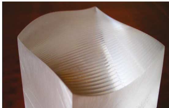
Figure 9. Manufactured freeform surface using CNC machining.
