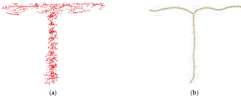
Figure 10. (a) An MMS point cloud imported in the L_1 -medial skeleton viewer. (b) Skeleton results (grey points are the input point cloud, green points are the nodes, and red lines are segments).
