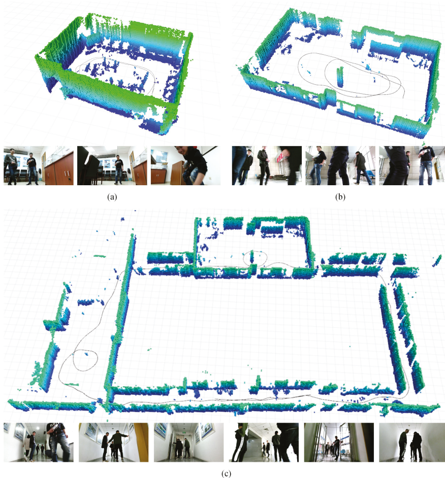
Figure 13. Results of the extension tests. (a) 8 \text{ m} \times 6 \text{ m} office (Voxel size: 0.05 m), (b) 15 \text{ m} \times 9 \text{ m} hall (Voxel size: 0.05 m), and (c) 37 \text{ m} \times 27 \text{ m} corridor (Voxel size: 0.1 m). The black lines are the robot trajectories of keyframes.
