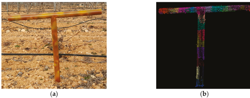
Figure 9. (a) VSAO; (b) example of a clustering TLS point cloud with the convex hull cluster algorithm.
