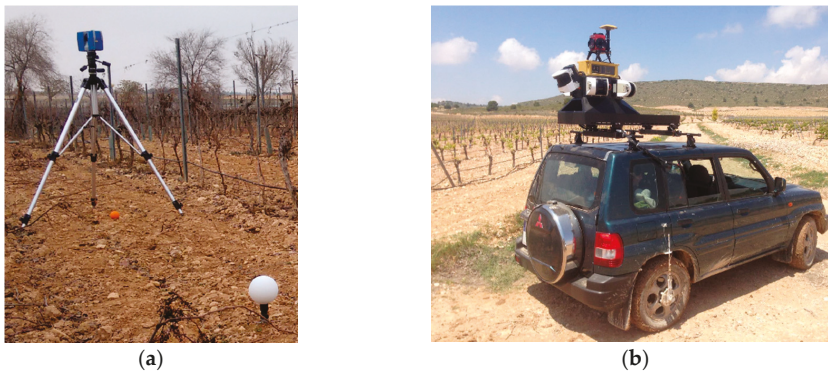
Figure 4. Laser scanner equipment. (a) A TLS mounted on a tripod with a head and calibrated sphere. (b) The MMS operating on a 4 × 4 vehicle.
