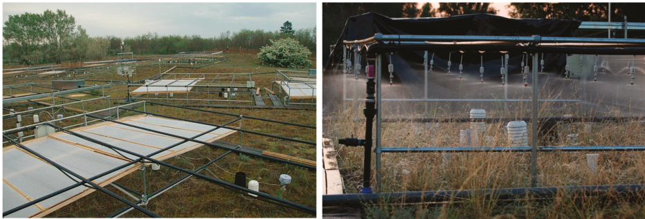
Figure 2. Left picture shows the removable plastic roofs used to exclude from rainfall for drought treatments in the ExDRain experiment and right picture the irrigating event for the watered plots.
