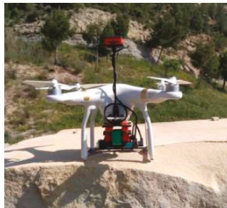
Figure 3. Phantom 3 DJI with the Parrot SEQUOIA camera and irradiance sensor, used for the aerial survey.
