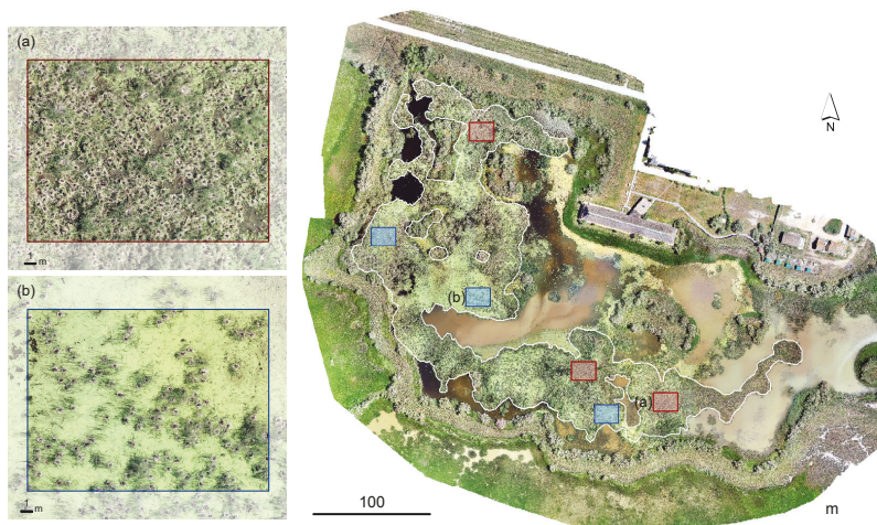
Figure 4. Orthomosaic image of high-resolution of the Glossy ibis colony in “Lucio de la FAO”. Image was mosaicked with Pix4D mapper Pro (Pix4D, Switzerland) after acquiring 448 photos through automatic flight of Phantom 4 Pro quadcopter (DJI Innovations, Shenzhen, China) on 14 May 2018. Squares show validation areas to test the accuracy of the automatic nest counting method to the visually nest count by an expert. Blue squares show densely macrophytes area ( Typha spp) whereas red squares show free areas of emergent vegetation covered by Lemna aquatic plant. White line delineates the Glossy ibis nesting area.
