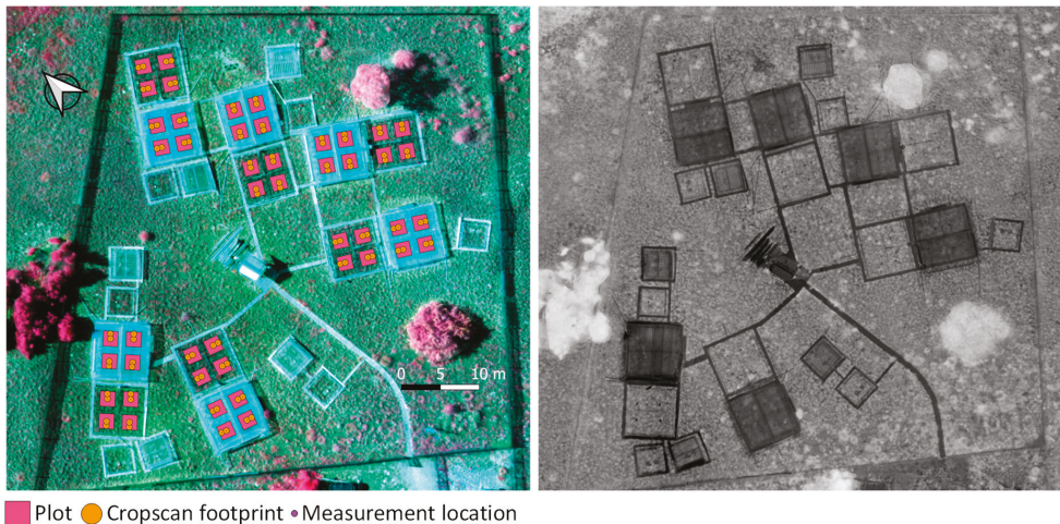
Figure 4. Left image shows a false color RGB composite with near infrared-red edge-red Sequoia bands with the overlay of plot limits, Cropscan sampling footprints and measurement location points. Right image shows Normalized Difference Vegetation Index (NDVI) image calculated with Sequoia near infrared and red bands evidencing the plots covered by plastic (darker plots).
