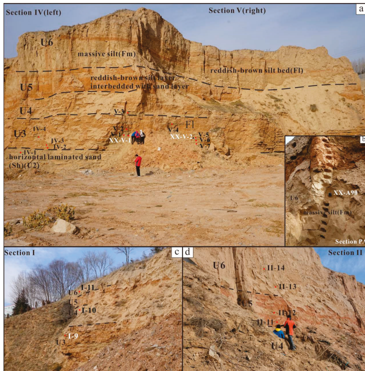
Figure 12. Sedimentary features of U6 in section IV and V, showing detailed sampling points. The dashed lines are the boundaries of the sediment units.
