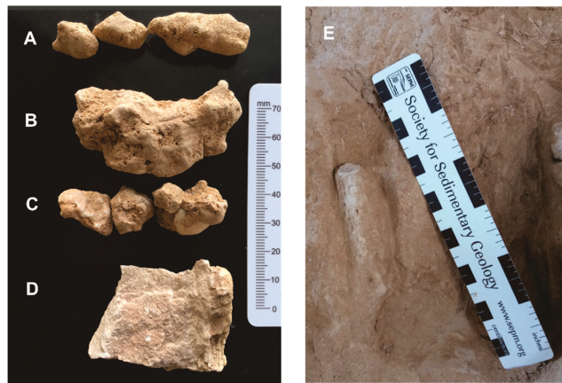
Figure 5. Examples of calcium carbonate concretions occurring in the coarse silts of T6: (A) three concretions collected, respectively, from depths of 3.56, 3.57 and 3.60 m; (B) a 2.5 cm thick concretion, obtained from a depth of 3.91–3.93 m; (C) two concretions and an agglomerate of two quartz pebbles, collected from a level at a depth of 4.73–4.83 m; (D) fragment of a quite continuous caliche level, 3 cm thick, that occurs at a depth of 5.33–5.36 m; (E) a 1 cm thick rhizolith, collected from a depth of 3.91–3.93 m.
