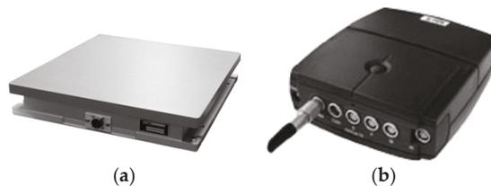
**Figure 1.** The experimental instruments. (a) AMTI force plate (AMTI<sup>®</sup>, Watertown, MA, USA) and (b) NeXus-10 physiological monitoring system (Mind Media<sup>®</sup>, BV, Herten, The Netherlands).
