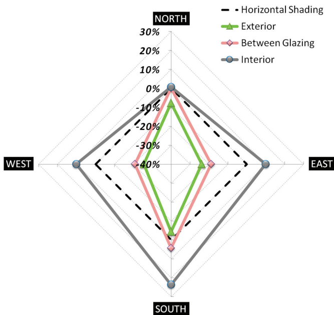
Figure 12. Saving ratio of the heating and cooling load according to the type of shading (WWR 80%, U-value: 2.1, SHGC: 0.4).
