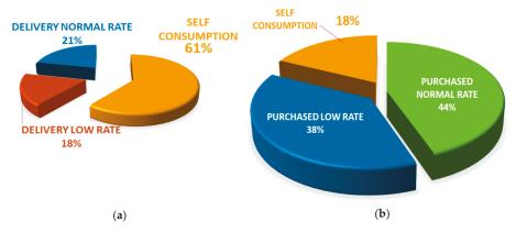
Figure 2. PowerMatching City electricity purchase, self-consumption, and production in 2012: (a) Electricity generated by PV and  $\mu$ CHP; percentages of self-consumption and electricity delivery depending rates; (b) Self consumption and electricity purchased from the grid, with purchase percentages depending on rates.
