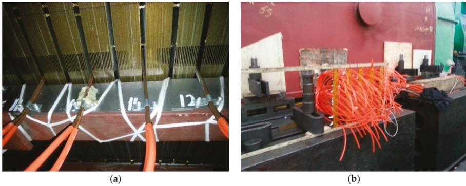
**Figure 2.** Placement and measuring position of pitot tube in the stator ventilation ducts. (a) Placement position of pitot tube; (b) measuring position of ventilation duct.
