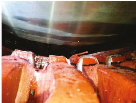
**Figure 3.** The sensor placement at the air gap entrance.
