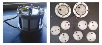
Figure 3. Electrolyser (left) and, steel electrodes used in the electrolyser unit (right).
