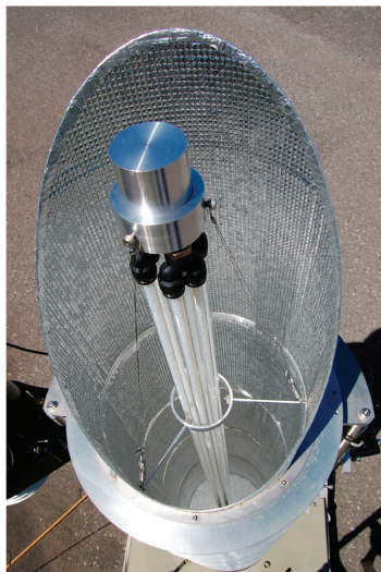
Figure 11. Top view of the HQC21-packed glass tube reactor.
