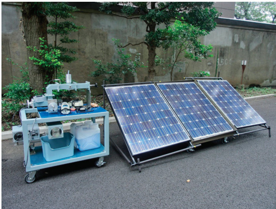
Figure 13. Water sterilization equipment used to sterilize rain water samples using the solar cells located on the right hand side of the photograph and the TiO 2 -coated MDELs (150 pieces) [55].
