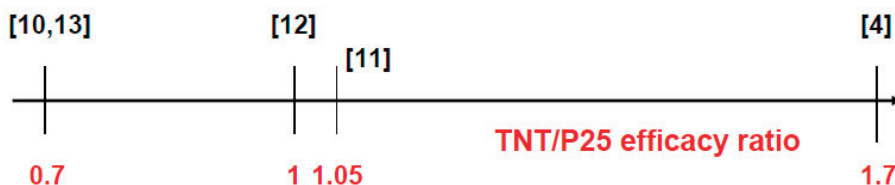
Figure 4. TNT/P25 TNP efficacy ratio in the photocatalytic removal of toluene [4,10,11] or acetaldehyde [12,13]. The corresponding references are indicated in brackets.
