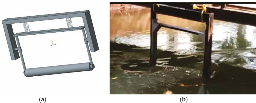
Figure 13. (a) Model of HVPG; (b) field test at Palissery irrigation canal for m^* = 0.66 and U_r = 4, 8, and 12.
