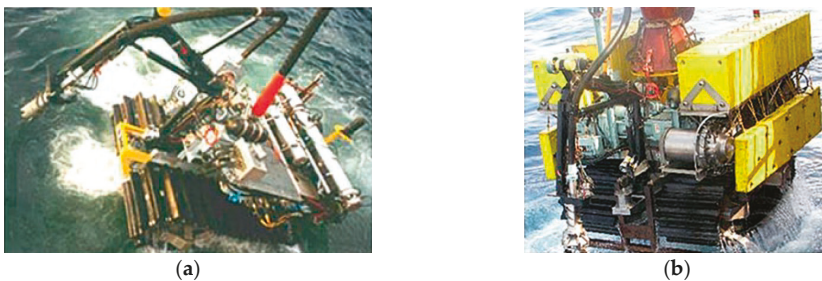
Figure 2. (a) Underwater mining system with manipulator and cutter for 500 m water depth; (b) Enhanced underwater mining system for 500 m water depth [33].
