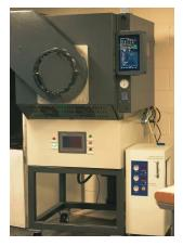
Figure 1. Hydrogen oven and H<sub>2</sub> generator.
