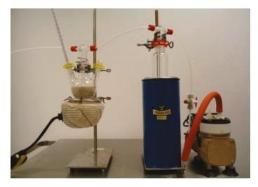
Figure 4. Condensation unit for the recovery of [<sup>18</sup>O]-water from azeotropic mixtures.
