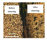
Figure 8. Micrography of polished samples before and after sintering at (800 °C).
