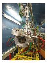
Figure 2. Targetry "hatch tip" low current (<2 µA) for development.
