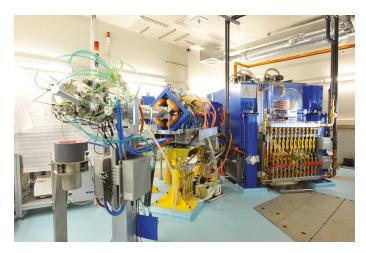
**Figure 3.** The TR-Flex cyclotron at the HZDR. The beamline 1B with a 4-port target selector is shown in the foreground. The second 4-port target selector is at the opposite side of the Cyclotron. Picture: HZDR/Frank Bierstedt.
