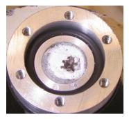
Figure 5. Photograph of BNNT material in the prototype target, showing material damage resulting from irradiation at  $20-\mu$ A beam current.
