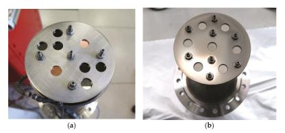
Figure 2. Masks assembled on heated substrate-holder for Mo sputtering (a) and on nonheated substrate-holder for Y sputtering (b).
