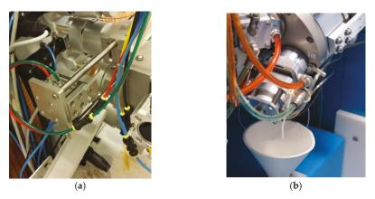
**Figure 3.** Solid target stations used for under-beam target tests: (**a**) TEMA Synergie target station prototype of PETtrace cyclotron (S. Orsola-Malpighi Hospital, Bologna); (**b**) TR19 cyclotron target station (Sacro Cuore Hospital, Negrar, Verona).
