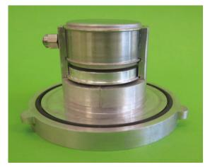
Figure 6. The tandem Rb/Ga targets mounted on a bayonet-mount plug.
