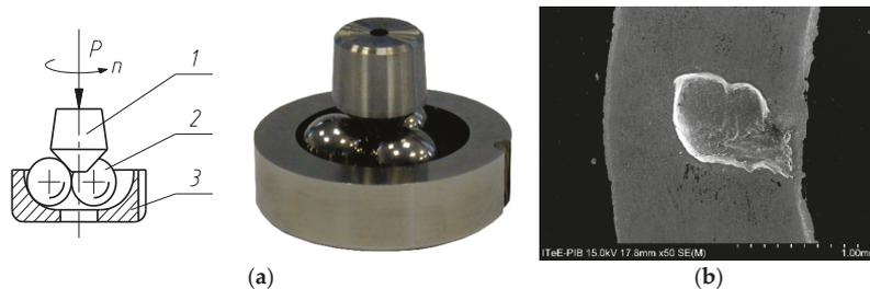
**Figure 2.** (a) Cone-balls tribosystem: 1—cone, 2—balls, 3—race; (b) SEM image of a typical pit on the cone.
