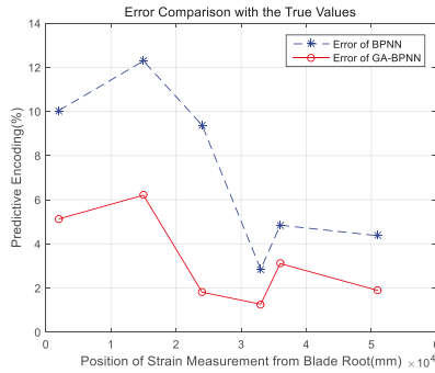
Figure 7. The comparison results of prediction errors for the center of suction side.
