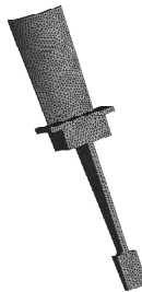
Figure 5. Finite element (FE) model of turbine blisk.
