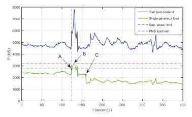
Figure 11. System behavior during a power peak.
