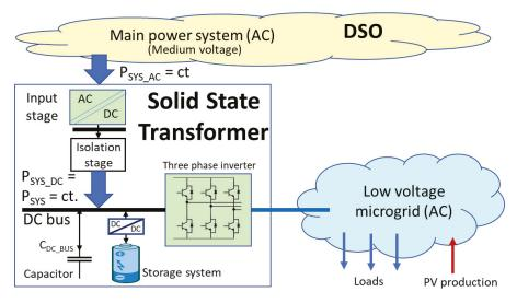
Figure 5. The basic configuration of the proposed SST.
