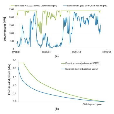
**Figure 1.** Comparison of the time series for power production based on actual wind and performance data from a wind farm in Germany (**a**) and generalized feed-in duration curves for baseline and advanced wind energy converters (WEC) (**b**).
