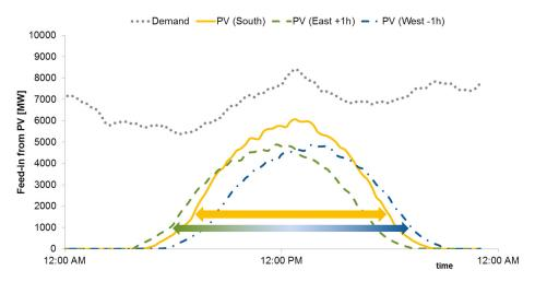
Figure 2. Comparison of normalized baseline feed-in (PV(S) vs. modified advanced feed-in PV (E) and PV (W) installations over 24 h.
