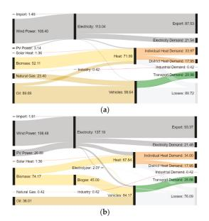
Figure 1. Sankey diagrams of energy flows in GWh for Samsø for 2015 (a) and 2030 (b) [32].
