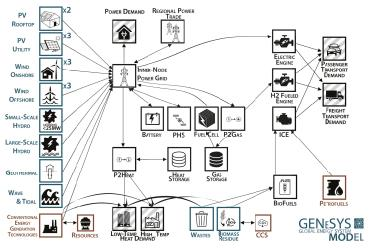
Figure 1. Structure of GENeSYS-MOD v2.0.
