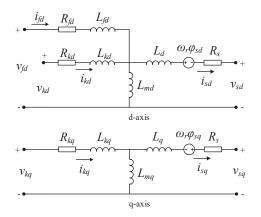
Figure 7. Equivalent circuit of synchronous generator block in a *dq* reference frame.
