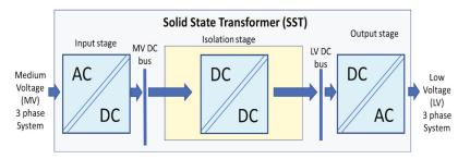
Figure 1. Solid state transformer design example.
