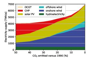
Figure 6. Breakdown of electricity supply by technology.
