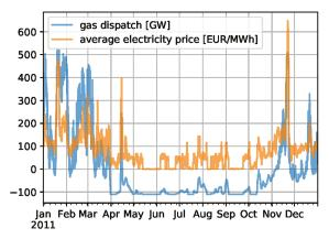
**Figure 11.** Zero CO<sub>2</sub> scenario: Methane dispatch (positive when synthetic methane is consumed, negative when produced by methanation) versus average electricity prices.
