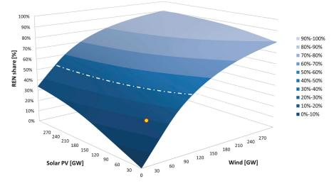
Figure 6. REN share surface plot for Case A, including the 2017 capacities from wind and solar PV (point marking), and the 50% REN share marking for various combinations resulting in a 50% REN share (mixed dotted-dashed line).
