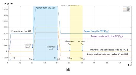
**Figure 8.** Simulations results in Scenario 1. (a) DC bus voltage in the SST; (b) Current injected from the main grid in the DC bus of the SST; (c) The output currents of the SST (ISST), injected into the microgrid; (d) Active power evolution in different parts of the AC microgrid.
