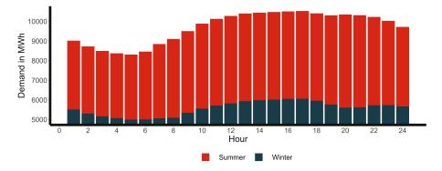
Figure 3. Load profile of the Mexican electric system.
