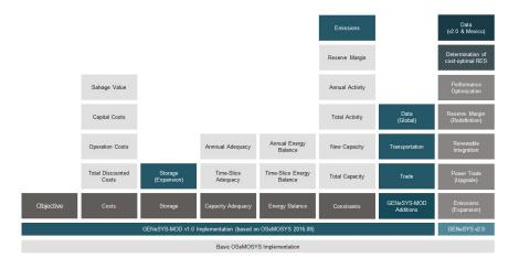
Figure A1. Model structure of the GENeSYS-MOD implementation used in this study.
