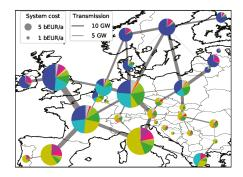
Figure 1. Costs by country with zero CO<sub>2</sub> emissions and optimal transmission. The colour assignments follow Figure 3.
