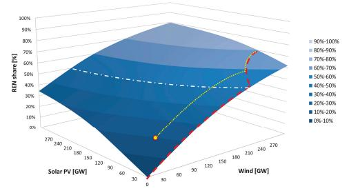
**Figure 9.** REN share surface plot and efficient pathway for Case BS, including the efficient pathway starting at 0 GW wind and solar PV deployment (dashed line), the efficient pathway starting at the 2017 capacities from wind and solar PV (dotted line), and the 50% REN share marking for various combinations resulting in a 50% REN share (mixed dotted-dashed line).
