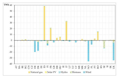
Figure 11. Change in electricity generation in 2050 due to lower connectivity levels.
