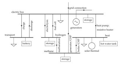
**Figure 2.** Energy flow at a single node. In this model, a node represents a whole European country. Within each node, there is a bus (thick horizontal line) for each energy carrier (electric, transport, heat, hydrogen, and methane), to which different loads (triangles), energy sources (circles), storage units (rectangles), and converters (lines connecting buses) are attached. The lines with arrows show the direction of energy transfer (Source: [29]).
