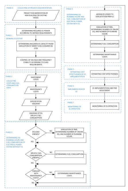
Figure 14. Block diagram of the ES implementation process.
