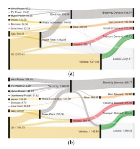
Figure 3. Sankey diagrams of energy flows in GWh for Madeira for 2014 (a) and 2030 (b) [32].
