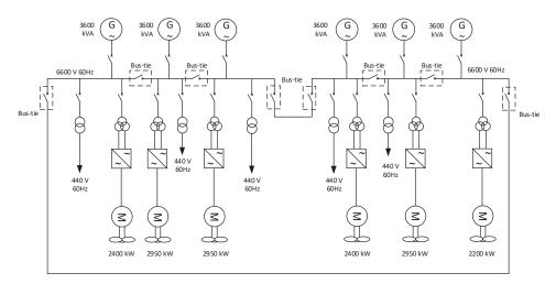
Figure 1. Typical topology of a dynamically positioned (DP) vessel electrical power system.
