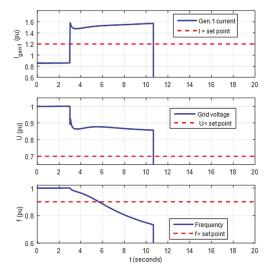
Figure 8. Simulation results for one DG loss without ES.
