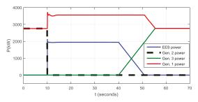
Figure 10. Simulation scenario for 3.6 MVA generator loss when two DGs are running in parallel, each loaded with 95% of nominal power.
