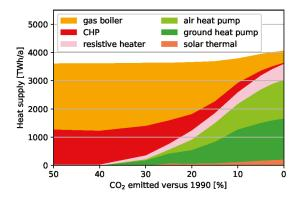
Figure 7. Breakdown of space and water heating supply by technology.
