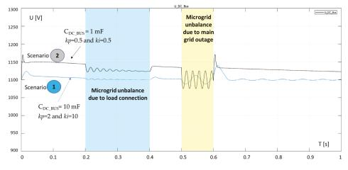
Figure 10. Superposition of the SST DC bus voltage variation in both scenarios (1 and 2).
