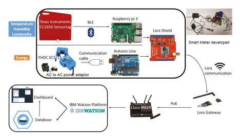
Figure 4. Smart meters for electricity measurement and a temperature/luminosity sensor with a Lora network, sending data to IBM Watson.
