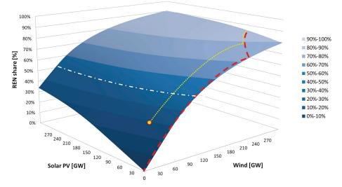
**Figure 10.** REN share surface plot and efficient pathway for Case AS, including the efficient pathway starting at 0 GW wind and solar PV deployment (dashed line), the efficient pathway starting at the 2017 capacities for wind and solar PV (dotted line), and the 50% REN share marking for various combinations resulting in a 50% REN share (mixed dotted-dashed line).
