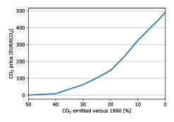
**Figure 4.** CO<sub>2</sub> shadow price in the model as CO<sub>2</sub> emissions are restricted in the case of cost-optimal cross-border transmission.
