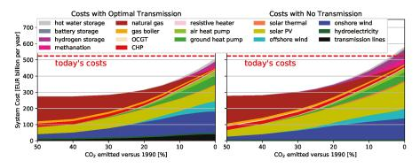
**Figure 3.** System costs for electricity, land transport, and space and water heating in Europe with a changing  $CO_2$  limit, assuming the 2030 cost projections from Table 1. Left is the case with cost-optimal transmission, right is with no transmission. Estimated costs for today's system are marked with a red dashed line.
