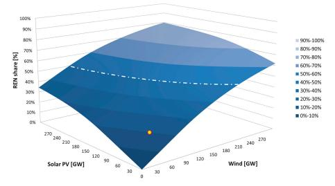
**Figure 4.** REN share surface plot for Case B, including the 2017 capacities from wind and solar PV (point marking), and the 50% REN share marking for various combinations resulting in a 50% REN share (mixed dotted-dashed line).
