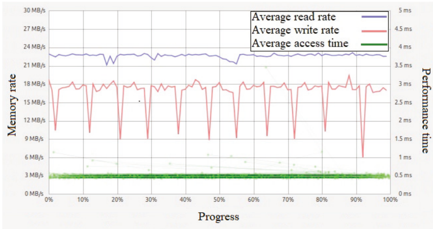
Figure 9. Comparison between read and write performance of SD card on RP3.
