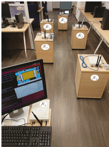
Figure 7. An experimental setup for a D2D route with five hops using RP3 in the RPU testbed, which is equivalent to Figure 4b.
