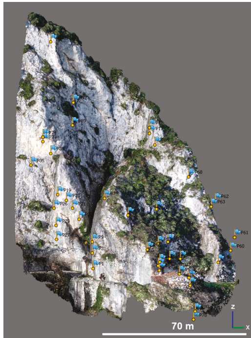
Figure 2. Perspective view, from SE, of Ground Control Point (GCP) spatial distribution along the slope (dense 3D textured point cloud in background).
