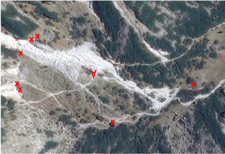
Figure 5. Geodetic network (crosses mark the points of geodetic network and the arrow indicates the position of the total station. Source of map: maps.google.com).
