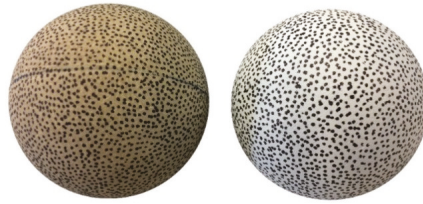
Figure 2. Ball preparation. Left: pressurised ball core; Right: pressureless ball core.
