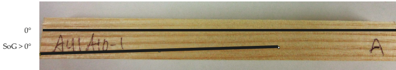
Figure 3. Example of a radial slope-of-grain measurement.
