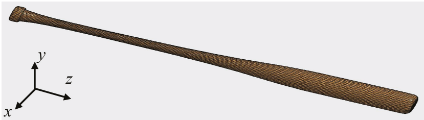
Figure 6. Finite element model of a C243 bat.
