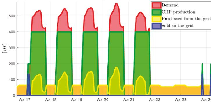
Figure 8. Optimal operation: electric demand and load sharing in a typical week.
