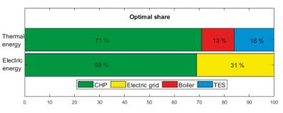
Figure 7. Optimal electric and thermal load sharing.
