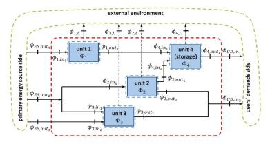
Figure 1. General configuration of a fleet of energy units.
