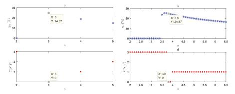
Figure 10. Variation of global exergy efficiency and number of violated constraints with number of compression stages (a,c) and compressor pressure ratio (b,d) at optimal point.
