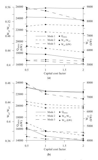
**Figure 7.** (a) Effect of capital cost on the optimal values of  $\dot{Q}_{HRSG}$  and  $\dot{W}_{ST}$  and on the fraction  $\dot{W}_{ST}/\dot{W}_{GT}$  with MDO. (b) Effect of capital cost on the optimal values of  $\dot{Q}_{HRSG}$  and  $\dot{W}_{ST}$  and on the fraction  $\dot{W}_{ST}/\dot{W}_{GT}$  for natural gas.
