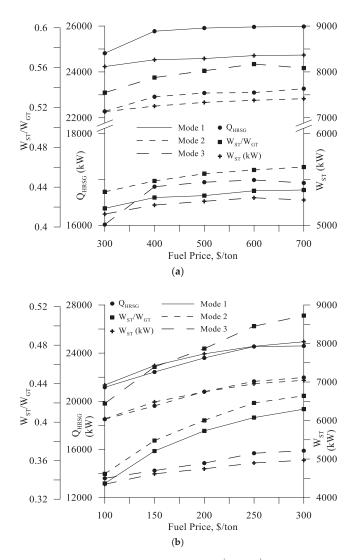
**Figure 6.** (a) Effect of MDO price on the optimal values of  $\dot{Q}_{HRSG}$ ,  $\dot{W}_{ST}$  and (b) the effect of natural gas price on the optimal values of  $\dot{Q}_{HRSG}$ ,  $\dot{W}_{ST}$ , and  $\dot{W}_{ST}/\dot{W}_{GT}$ .
