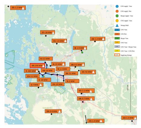
**Figure 4.** Optimal supply network in Case 1 with storages (triangles) and pipelines (blue lines). The type of fuel used is denoted by color in the rectangles, which also reports the fuel demand. The node number is given by the bold number in the rectangle. The node with the storage supplying regasified LNG into the pipeline is denoted by the red framed rectangle (Background map source: © OpenStreetMap contributors).
