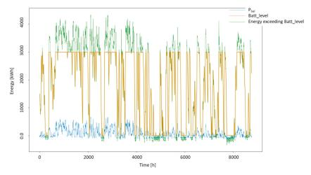
**Figure 12.** 4 Weptos configuration. Power balance during 8760 hours from 1 September 2016 to 31 August 2017. Pbal = Pprod – Pcons (blue), Batt\_level: battery stored energy (orange), Energy Exceeding Batt\_level (green): the energy that cannot be stored in the batteries, either because batteries are already full or because there is not enough energy to be stored, as it is all used for the demand.
