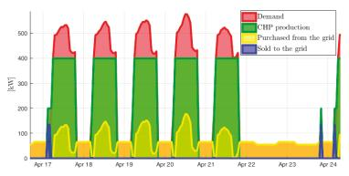
Figure 8. Optimal operation: electric demand and load sharing in a typical week.
