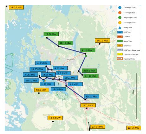
Figure 3. Optimal supply chain for the Base Case. The fuel supplied to the nodes is indicated in the colored boxes (Background map source: © OpenStreetMap contributors).
