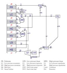
Figure 4. Bottoming cycle and internal structure of the HRSG.
