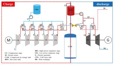
Figure 1. Schematic diagram of the proposed system.
