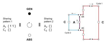
**Figure 4.** An example of topology definition of a basic configuration, including two elementary cycles and one absorption/generation process. (red line—refrigerant, blue line—absorbent solution).
