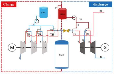
Figure 7. Schematic diagram of optimized system.
