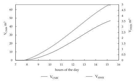
**Figure 6.** Off-design simulation of the charging phase (Reference day of May in Crotone)—volume increase in the storage sections: HWR (V<sub>HWR</sub>) and CMR (V<sub>CMR</sub>).
