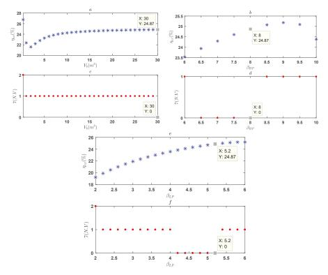
**Figure 11.** Variation of global exergy efficiency and number of violated constraints with volume of air storage tank (**a**,**c**), pressure ratio of high-pressure expansion stage (**b**,**d**) and low-pressure expansion stage (**e**,**f**) of pneumatic motor at optimal point.
