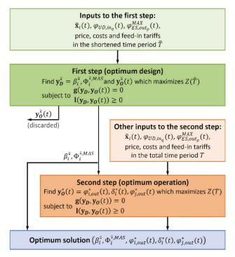
Figure 4. Two-step decomposed optimization procedure.
