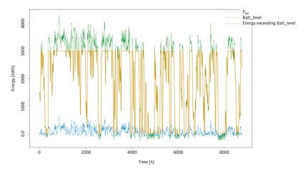
**Figure 8.** 2 Weptos configuration. Power balance during 8760 hours from 1 September 2016 to 31 August 2017. Pbal = Pprod – Pcons (blue), Batt\_level: battery stored energy (orange), Energy Exceeding Batt\_level (green): the energy that cannot be stored in the batteries, either because batteries are already full or because there is not enough energy to be stored, as it is all used for the demand.
