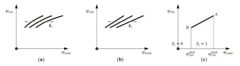
**Figure 2.** Characteristic map of an energy conversion unit having one fuel ( $\varphi_{i,in}$ ) and one product ( $\varphi_{i,out}$ ): (**a**) nonlinear input–output relationship, (**b**) linearized input–output relationship and (**c**) use of a binary variable  $\delta_i$  to identify the on/off status of the unit.
