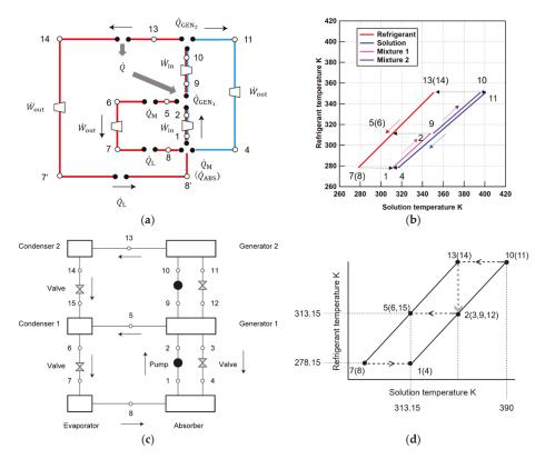
**Figure 10.** Optimal solution in case Y (red line—refrigerant, blue line—absorbent solution): (a) Basic configuration calculated; (b) Operating properties calculated; (c) Cycle configuration of an existing double-effect absorption refrigerator; (d) Operating properties of an existing system.
