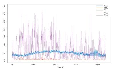
**Figure 6.** Power consumption, Power production and Power per meter of wave crest (Pcons, Pprod and Pwave) in kW for 2016, 4 Weptos configuration.
