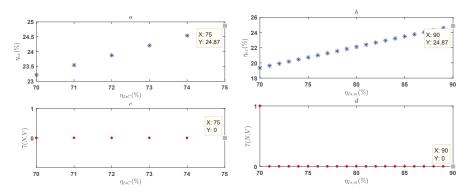
Figure 13. Variation of global exergy efficiency and number of violated constraints with compressor (a,c) and pneumatic motor (b,d) isentropic efficiency at optimal point.
