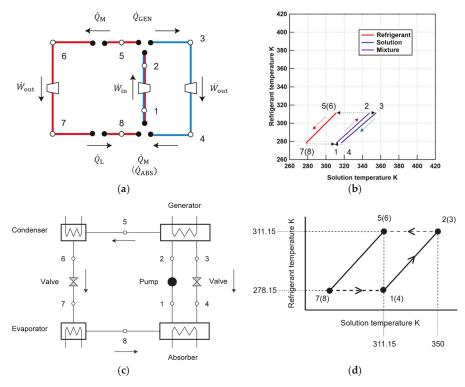
**Figure 9.** Optimal solution in case X (red line—refrigerant, blue line—absorbent solution): (**a**) Basic configuration calculated; (**b**) Operating properties calculated; (**c**) Cycle configuration of an existing single-effect absorption refrigerator; (**d**) Operating properties of an existing system.
