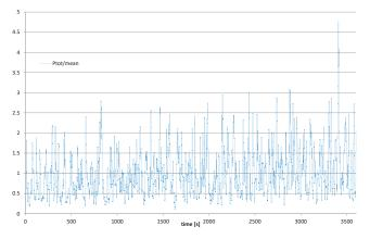
**Figure 13.** Illustration of short-term variability of produced power given in terms of normalized power (instantaneous power divided by the one-hour average) as function of time. Top: A full hour record, bottom: A zoom of the last 10 min where largest peak occurs.
