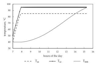
Figure 5. Off-design simulation of the charging phase (Reference day of May in Crotone)—temperature profile for the solar-thermal field and temperature increase of water in the IHR tank.
