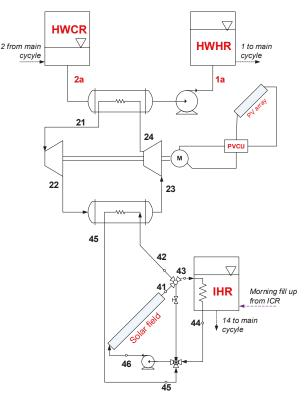
Figure 1. Solar-assisted heat pump cycle-schematic.
