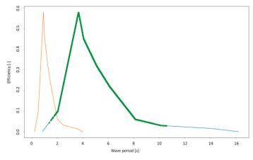
Figure 9. Efficiency of a Weptos with 3.96 m rotors diameter over different wave periods (green) and in the laboratory (yellow).
