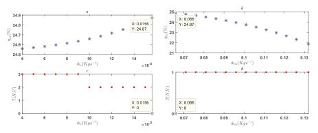
**Figure 15.** Variation of global exergy efficiency and number of violated constraints with compressor (**a**,**c**) and pneumatic motor (**b**,**d**) mass flow rate at optimal point.
