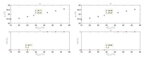
**Figure 12.** Variation of global exergy efficiency and number of violated constraints with inlet temperature of high-pressure (**a**,**c**) and low-pressure (**b**,**d**) expansion stages of pneumatic motor at optimal point.
