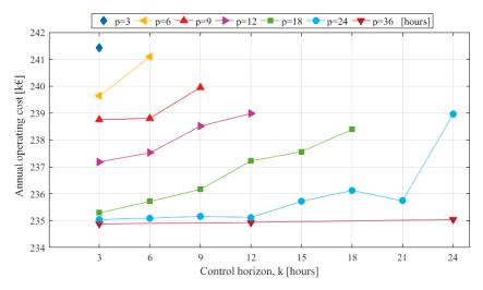
Figure 6. Impact of the prediction and control horizon lengths on the annual operating cost.
