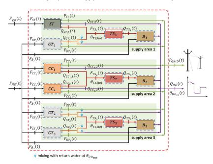
Figure 9. Fleet of large-scale energy units serving a district heating network.
