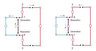
**Figure 2.** Examples of the basic configuration for the absorption system that is obtained by assembling two elementary cycles, in which each elementary cycle shares a part of compression(left)/expansion(right) process. (red line—refrigerant, blue line—absorbent solution).
