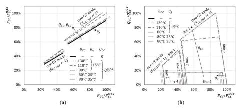
**Figure 8.** Characteristic maps of the CHP combined cycle unit (*CC*) for different generation ( $\theta_{CC}$ ) and ambient ( $\theta_A$ ) temperatures: (**a**) F - P for  $Q_{CC} = 0$  and  $Q_{CC} = Q_{ST}^{MAX}$  (**b**) Q - P map. For simplicity, the dependence on  $\theta_A$  is shown only for  $\theta_{CC} = 80^{\circ}$ .
