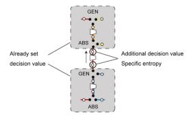
**Figure 7.** An example of topologies that require definition of several additional design parameters. (red line—refrigerant, blue line, yellow line—absorbent solution).
