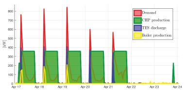
Figure 9. Optimal operation: thermal demand and load sharing in a typical week.
