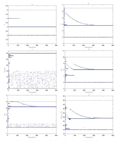
**Figure 8.** Scattering of optimal design variables during evolution; the case of the number of compression stage (**a**), of the compression pressure ratio (**b**), of the volume of air storage tank (**c**), of the pressure ratio of the high-pressure expansion stage (**d**), of the pressure ratio of the low-pressure expansion stage (**e**) and of the inlet temperature of the high-pressure expansion stage (**f**).
