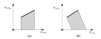
**Figure 3.** Additional characteristic maps of an energy conversion unit having more products: (a) the additional product ( $\varphi_{i,out_q}$ ) is generated by recovering waste streams, (b) the additional product ( $\varphi_{i,out_q}$ ) is generated consuming a part of the streams used to generate the main product ( $\varphi_{i,out_1}$ ).
