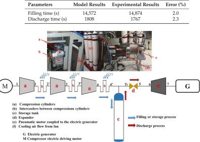
Figure 4. Global view and diagram of pilot system.
