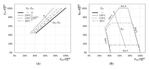
**Figure 7.** Characteristic maps of the CHP steam unit (*ST*) for different generation temperatures ( $\theta_{ST}$ ): (a) F - P map when  $Q_{ST} = 0$  and  $Q_{ST} = Q_{ST}^{MAX}$ , and (b) Q - P map.
