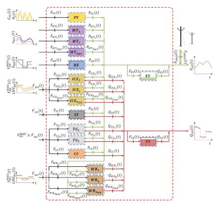
Figure 5. Fleet of units serving electrical and thermal energy users.
