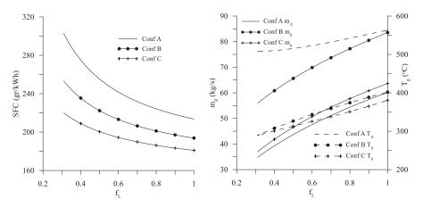
Figure 5. Variation of specific fuel consumption (SFC) and exhaust gas characteristics in partial load operation (fuel MDO).
