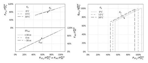
**Figure 6.** Characteristic maps of a CHP gas turbine (*GT*) for different ambient temperatures ( $\theta_A$ ): (**a**) *F* – *P* and (**b**) *Q* – *P* map. Figure 6a also represents the map of the hydroelectric unit (*HE*) for different available water head ( $\Delta h_{HE}$  is the difference between the off-design and design values of  $h_{HE}$ ).
