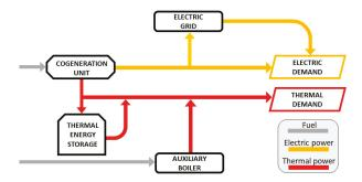
Figure 1. Schematic representation of the combined heat and power system.
