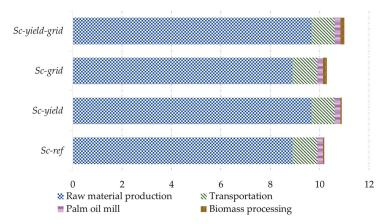
**Figure 8.** GHG emissions from a more efficient palm oil supply chain (MtCO<sub>2</sub>eq/y). Legend: *Sc-ref*: Incorporating the government policy to foster the utilization of palm biomass residue; *Sc-yield*: Improving the yield of small-scale plantations; *Sc-grid*: Improving bioelectricity delivery; *Sc-yield-grid*: Combination of *Sc-ref* and *Sc-grid*.
