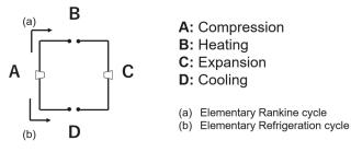
Figure 1. Basic configuration of elementary thermodynamic cycle.
