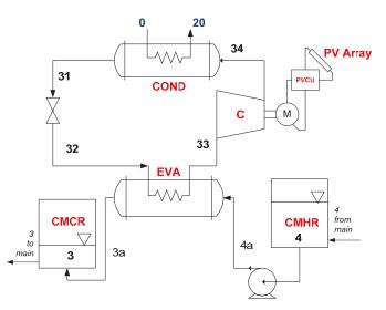
Figure 2. Refrigeration cycle—Schematic.
