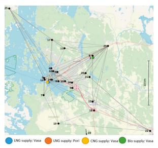
**Figure 2.** Network scheme with the location of the potential pipe connections (lines), customers (black dots) and suppliers (color dots). Node numbers are reported in red (Background map source: © OpenStreetMap contributors).
