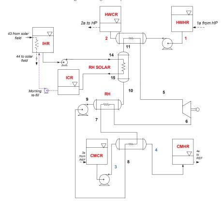
Figure 3. Trans-critical CO<sub>2</sub> power cycle—Schematic.
