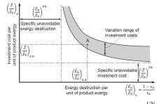
**Figure 3.** Definition of specific unavoidable exergy destruction  $(\dot{E}_{\rm D}/\dot{E}_{\rm P})_k^{\rm UN}$  and specific unavoidable investment cost  $(\dot{Z}/\dot{E}_{\rm P})_k^{\rm UN}$  based on the expected relationship between investment cost and exergy destruction (or exergetic efficiency) for the *k* th component. (Reproduced from [86]).
