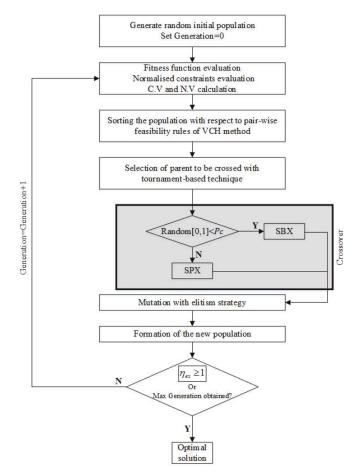
Figure 3. Proposed Real Coded Genetic Algorithm flow chart.
