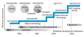
Figure 1. Technology development of pulverized coal power plants [9].
