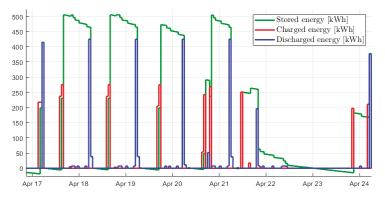
Figure 10. Optimal operation: TES stored, charged, and discharged energy in a typical week.
