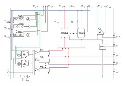
**Figure 8.** Superconfiguration of the generic energy system. (AB: auxiliary boiler; Cond: condenser; DGS: Diesel generator set; FWT: feed water tank, G: generator; HRSG: heat recovery steam generator; ME: main engine, ST: steam turbine).
