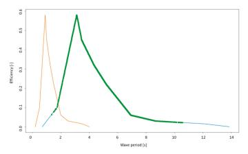
**Figure 5.** Efficiency of a Weptos with 3 m rotors diameter over different wave periods at location (green) and in the laboratory (yellow).
