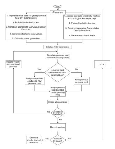
Figure 7. Flowchart of the Monte Carlo simulation and the Particle Swarm Optimization algorithm.
