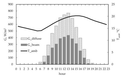
Figure 4. Distribution of meteorological data during the reference day of May in Crotone;  $T_{amb}$ —ambient temperature,  $G_{diffuse}$ —diffuse solar radiation,  $G_{beam}$ —direct solar radiation.
