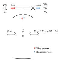
Figure 2. Schematic diagram of compression air storage tank.
