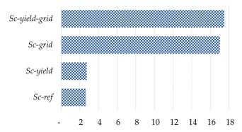
Figure 4. Total excess power to the grid (TWh/y). Legend: *Sc-ref*: Incorporating the government policy to foster the utilization of palm biomass residue; *Sc-yield*: Improving the yield of small-scale plantations; *Sc-grid*: Improving bioelectricity delivery; *Sc-yield-grid*: Combination of *Sc-ref* and *Sc-grid*.
