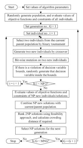
Figure 15. Flow chart of population-based NSGA-II algorithm.
