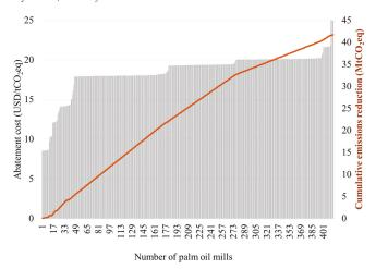
Figure 11. Technology abatement cost (bar chart, primary Y-axis) and cumulative emissions reduction (line, secondary Y-axis) of Sc-vield-grid.
