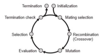
Figure 6. Flowchart of an evolutionary algorithm (adapted from [136]).
