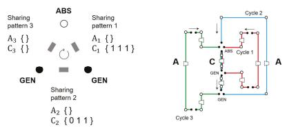
**Figure 5.** An example of topology definition of a basic configuration for the absorption system including three elementary cycles and one absorption process and two generation processes. (red line, green line—refrigerant, blue line—absorbent solution).
