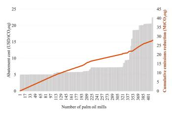
**Figure 10.** Technology abatement cost (bar chart, primary Y-axis) and cumulative emissions reduction (line, secondary Y-axis) of *Sc-ref*.
