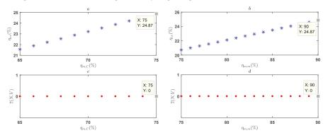
Figure 14. Variation of global exergy efficiency and number of violated constraints with compressor (a,c) and pneumatic motor (b,d) mechanical efficiency at optimal point.
