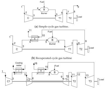
(c) Twin-spool intercooled recuperated-cycle gas turbine.
