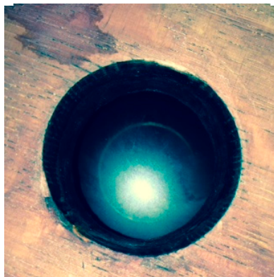
Figure 6. A thin film formed on top of the wine surface that influenced the ullage sensor reading.
