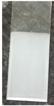
Figure 7. Representative appearance image of the coating aged for 5 days, obtained using a dipping velocity of 1000 mm/min.
