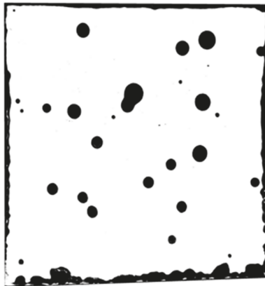
Figure 7. Binary image of Figure 8 to calculate the total corroded area.
