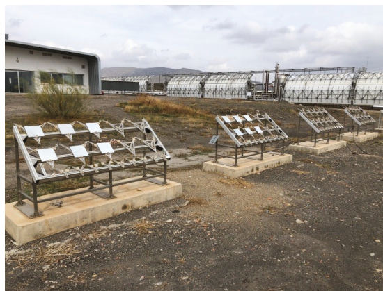
Figure 1. Exposure racks with mirror samples installed in south direction at the Plataforma Solar de Almería (PSA) facilities.
