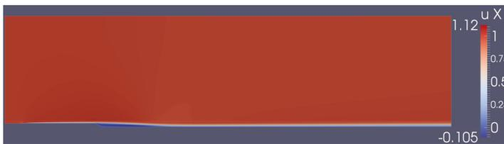
Figure 5. Horizontal component  $U$  of the base-flow velocity at  $Re = 1000$ .
