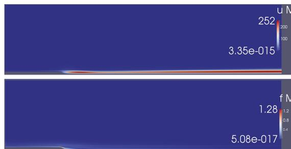
**Figure 10.** Magnitude of the optimal response and of the corresponding optimal forcing fields,  $|u''|$  and  $|f|$ , in the upper and lower panels, respectively, at  $Re = 1000$  and  $\beta = 1$ . The gain is maximized according to (7).
