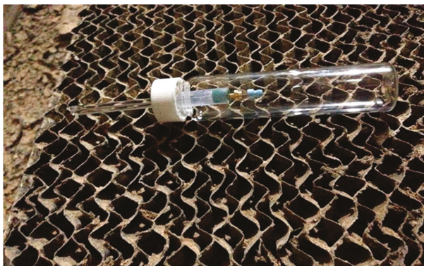
Figure 8. Field air sampling in TWA SPME mode on a commercial swine farm (Farm 2) in Iowa. The air sample diffuses through the opening in the GC glass liner (left side of the photo) onto an SPME fiber fully exposed inside the liner. A short section of Teflon tubing and a half-hole septum seal the liner and facilitate SPME insertion. A clear glass vial encloses the SPME assembly from dust and other gases in the sampled air.
