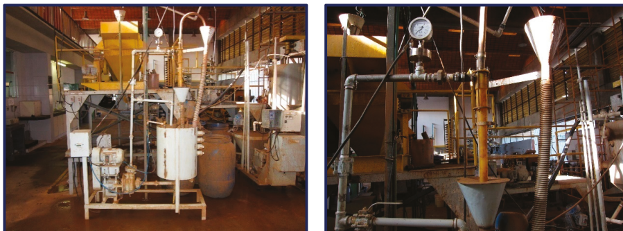
Figure 1. Apparatus for the desliming operation.
