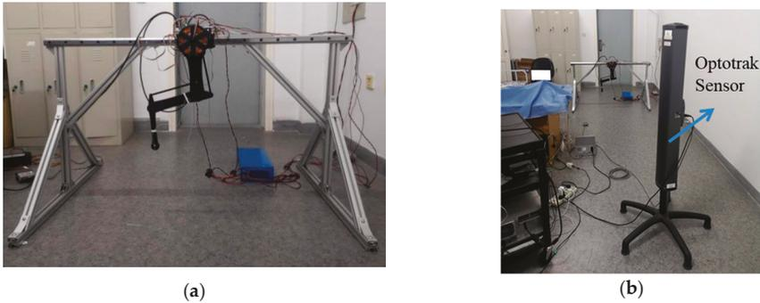
**Figure 18.** Experimental platform. (a) One leg experimental platform. (b) Trajectory measurement with Optotrak sensor.
