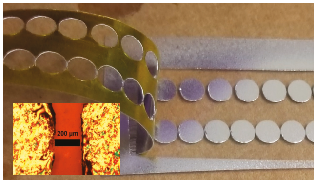
Figure 2. Spray-on Liquid-Metal electrode stencil removal process step. Inset: Magnified view of a liquid-metal electrode pair with a channel width of 200 \mu\text{m} .
