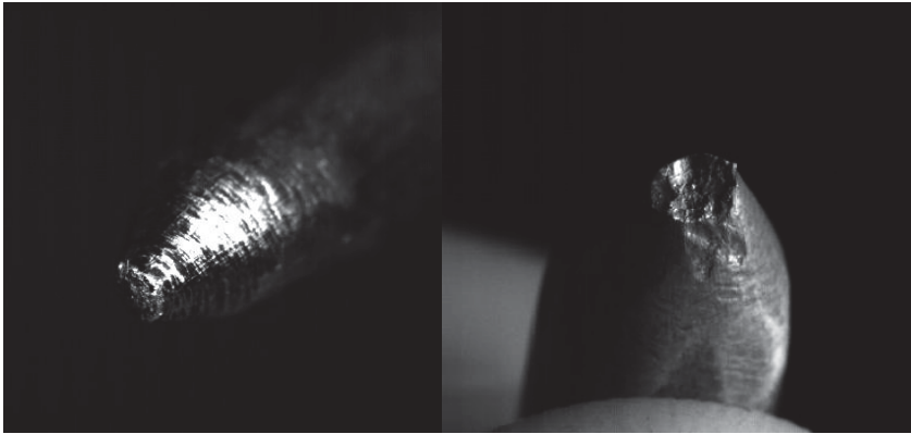
Figure 10. Photographs of the cathode (left) and anode (right) after the series of 15 experiments for I = 450 A. Diameter of both electrodes is 6 mm.
